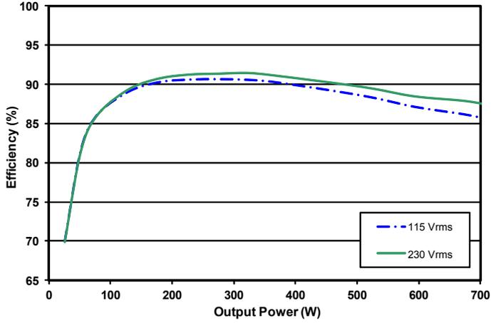
Figure 7: 48 V<sub>OUT</sub> efficiency curves.
