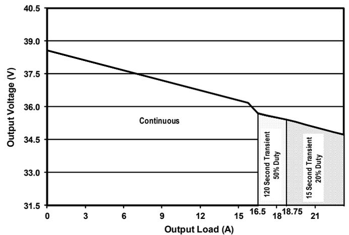
Figure 6: 36 V<sub>OUT</sub> droop characteristic.
