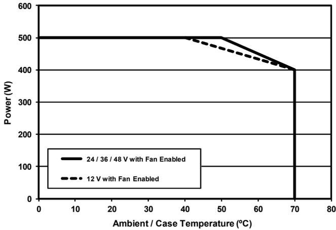
Figure 9: Continuous power derating curve in natural convection.
