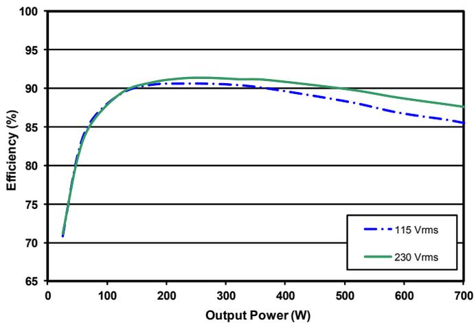
Figure 5: 36 V<sub>OUT</sub> efficiency curves.
