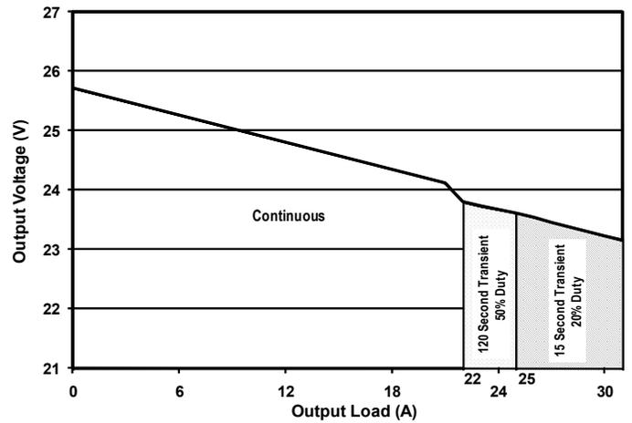
Figure 4: 24 V<sub>OUT</sub> droop characteristic.
