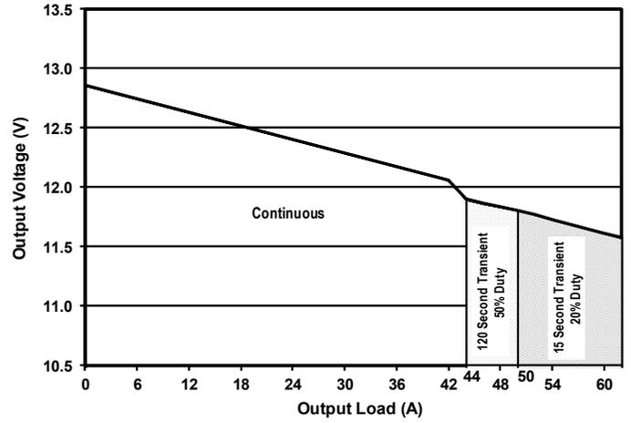
Figure 2: 12 V<sub>OUT</sub> droop characteristic.
