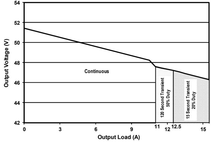
Figure 8: 48 V<sub>OUT</sub> droop characteristic.
