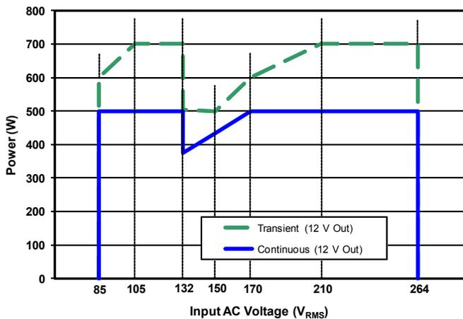
Figure 11: Rated output power vs Input AC Voltage.
