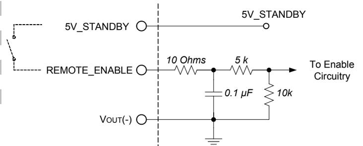
Figure C: Remote enable interface circuitry.
