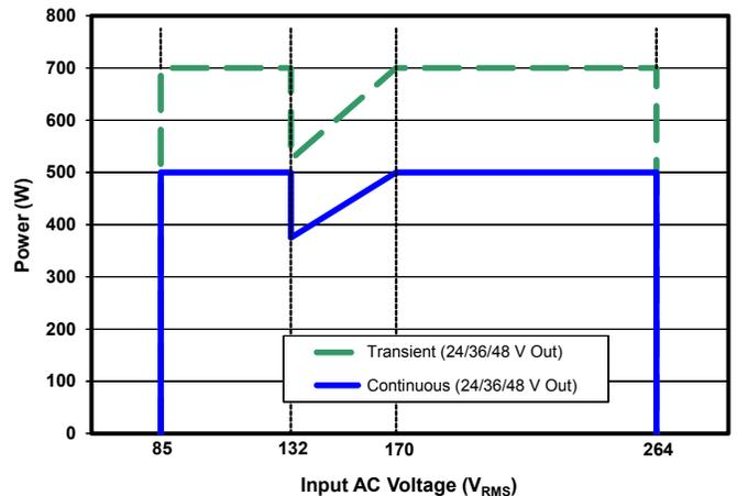
Figure 12: Rated output power vs Input AC Voltage.
