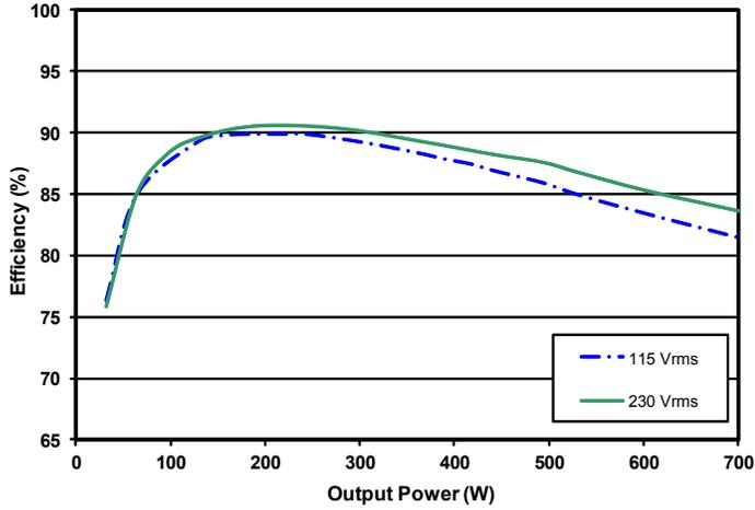
Figure 1: 12 V<sub>OUT</sub> efficiency curves.
