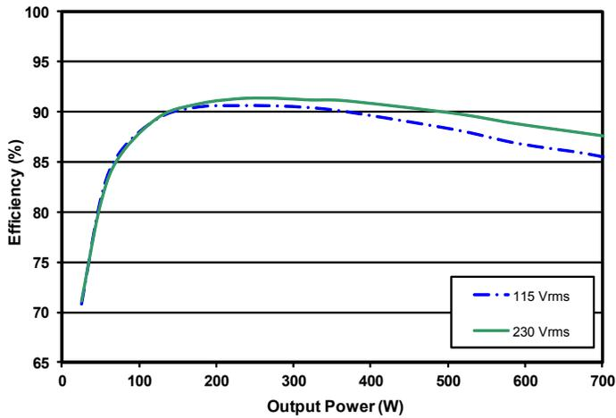
Figure 3: 24 V<sub>OUT</sub> efficiency curves.
