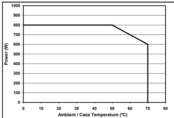
Figure 11: Continuous power derating curve in natural convection.
