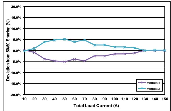
Figure I: Typical current share performance of 2 paralleled modules
