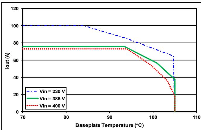
Figure 5: Maximum output current vs. baseplate temperature.
