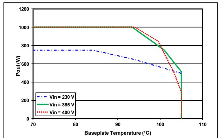
Figure 6: Maximum output power vs. baseplate temperature.
