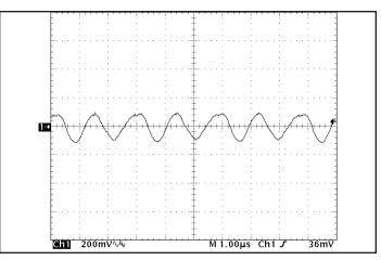
Figure 16: Output voltage ripple at nominal input voltage and rated load current (200 mV/div). Load capacitance: 1  $\mu$ F ceramic capacitor and 10  $\mu$ F tantalum capacitor. Bandwidth: 20 MHz. See Figure 13.
