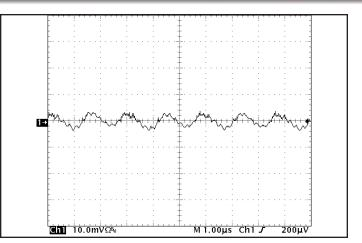
Figure 14: Input terminal ripple current, ic, at full rated output current and nominal input voltage with 10  $\mu$ H source impedance and 47  $\mu$ F ceramic capacitor (100 mA/div). See Figure 13.
