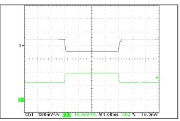
Figure 12: Output voltage response to step-change in load current (50%-75%-50% of lout(max):  $dI/dt = 1 A/\mu s$ ). Load cap: 10  $\mu$ F tantalum cap and 500  $\mu$ F ceramic capacitor bank. Ch 1: Vout (500 mV/div), Ch 2: lout (5 A/div).
