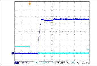
Figure 9: Turn-on transient at half load (resistive load) (10 ms/div). Load cap: 10 µF tantalum capacitor. Input voltage pre-applied. Ch 1: Vout (10 V/div). Ch 2: ON/OFF input (5 V/div).
