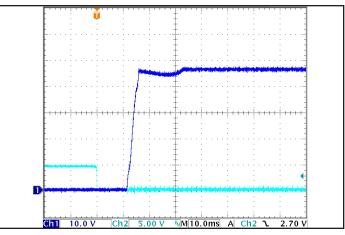
Figure 10: Turn-on transient at half load (resistive load) (10 ms/div). Load cap: 10 µF tantalum capacitor and 500 uF ceramic capacitor bank. Input voltage pre-applied. Ch 1: Vout (10 V/div). Ch 2: ON/OFF input (5 V/div).
