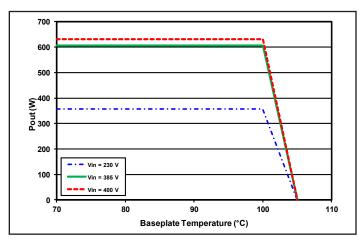
Figure 6: Maximum output power vs. baseplate temperature.
