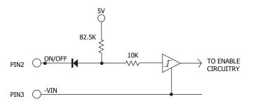
Figure B: Internal ON/OFF pin circuitry
