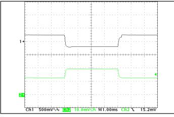
Figure 11: Output voltage response to step-change in load current (50%-75%-50% of lout(max);  $dI/dt = 0.1 A/\mu s$ ). Load cap: 10  $\mu$ F tantalum cap and 1  $\mu$ F ceramic cap. Ch 1: Vout (500 mV/div), Ch 2: lout (5 A/div).
