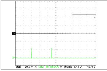
Figure 17:Rise of output voltage after the removal of a short circuit across the output terminals. Rshort =  $5 \text{ m}\Omega$ . Ch1: Vout (20 V/div). Ch 2: Iout (50 A/div). Bandwidth: 20 MHz.
