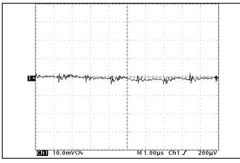
Figure 15: Input reflected ripple current, is, through a 10  $\mu$ H source inductor, using a 47  $\mu$ F ceramic input capacitor (5 mA/div). See Figure 13.
