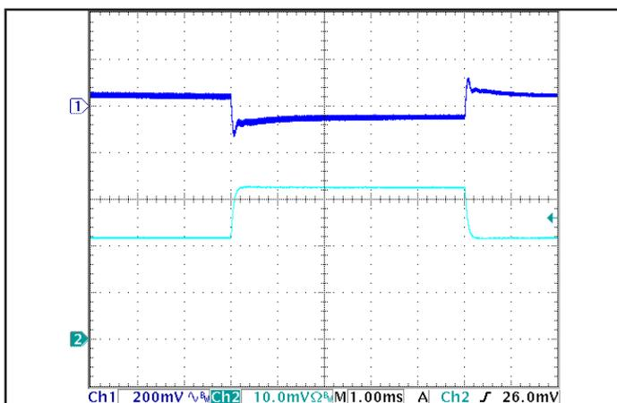
Figure 11: Output voltage response to step-change in load current (50%-75%-50% of I<sub>out</sub>(max); dI/dt = 0.1 A/μs). Load cap: 15 μF, 100 mΩ ESR tantalum cap and 1 μF ceramic cap. Top trace: V<sub>out</sub> (200 mV/div), Bottom trace: I<sub>out</sub> (10 A/div).
