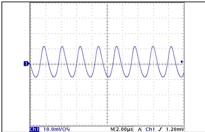
Figure 13: Input Terminal Ripple Current,  $i_c$ , at full rated output current and nominal input voltage with  $10\ \mu\text{H}$  source impedance and  $47\ \mu\text{F}$  electrolytic capacitor ( $50\ \text{mA/div}$ ). See Figure 12.
