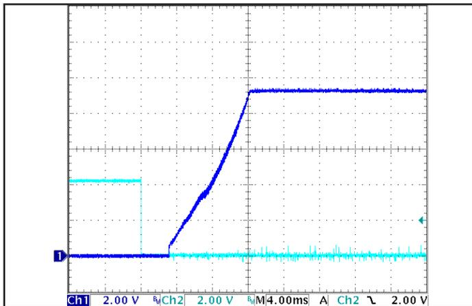
Figure 9: Turn-on transient at half load (resistive load) and 3 mF output capacitance (4.0 ms/div). Input voltage pre-applied. Channel 1: V<sub>out</sub> (2 V/div). Channel 2: ON/OFF input (2 V/div).
