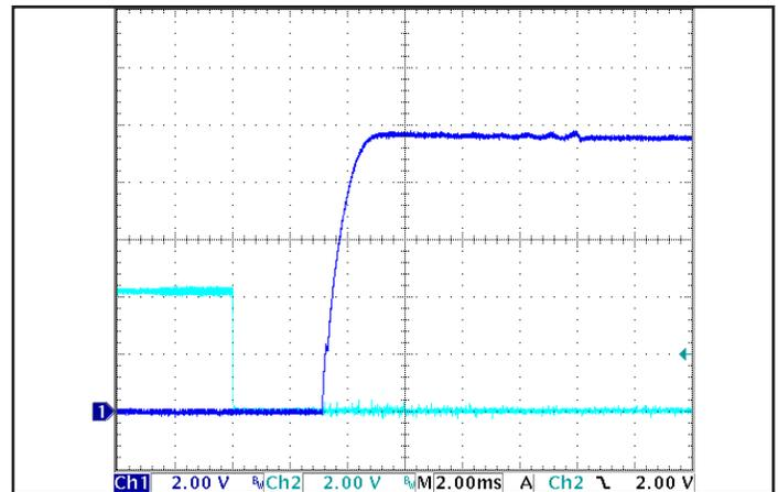
Figure 10: Turn-on transient at zero load and 3 mF output capacitance (2.0 ms/div). Input voltage pre-applied. Channel 1: V<sub>out</sub> (2 V/div). Channel 2: ON/OFF input (2 V/div).
