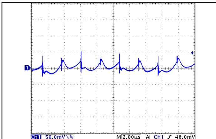
Figure 15: Output voltage ripple at nominal input voltage and rated load current ( $50\ \text{mV/div}$ ). Load capacitance:  $1\ \mu\text{F}$  ceramic capacitor and  $15\ \mu\text{F}$  tantalum capacitor. Bandwidth:  $20\ \text{MHz}$ . See Figure 12.
