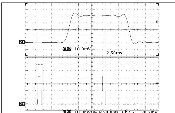
Figure 17: Load current ( $20\ \text{A/div}$ ) as a function of time when the converter attempts to turn on into a  $1\ \text{m}\Omega$  short circuit. Top trace ( $2.5\ \text{ms/div}$ ) is an expansion of the on-time portion of the bottom trace.
