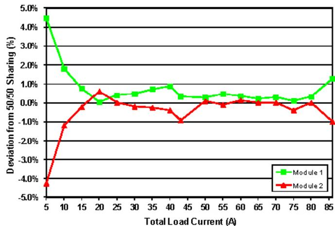
Figure I: Current share performance of 2 paralleled modules
