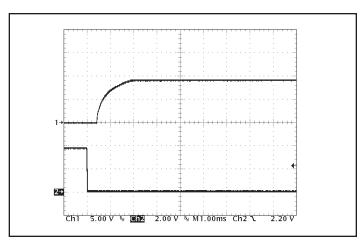
Figure 9: Turn-on transient at nominal input voltage and full load (resistive load) (1 ms/div). Load cap: 3 mF output capacitance. Input voltage pre-applied. Ch 1: Vout (5 V/div), Ch 2: ON/OFF input (2 V/div).
