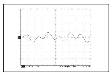
Figure 15: Input reflected ripple current at nominal input voltage and full rated current, is, through a 10  $\mu$ H source inductor, using a 47  $\mu$ F electrolytic input capacitor (20 mA/div).
