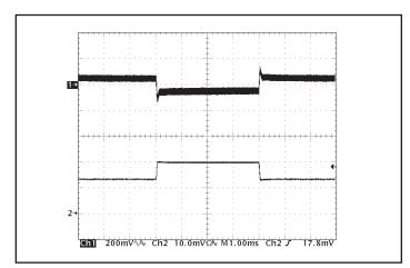
Figure 11: Output voltage response to step-change in load current (50%-75%-50% of lout(max);  $dI/dt=0.1~A/\mu s$ ). Load cap: 15  $\mu F$  tantalum cap and 1  $\mu F$  ceramic cap. Ch 1: Vout (200 mV/div), Ch 2: lout (10 A/div).
