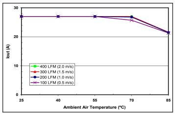
Figure 5: Maximum output power derating curve vs. ambient air temperature for airflow rates of 100 LFM through 400 LFM with air flowing from pin 1 to pin 3 (Vin = 48 V).
