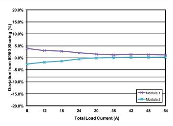
Figure 1: Current share performance of 2 paralleled modules
