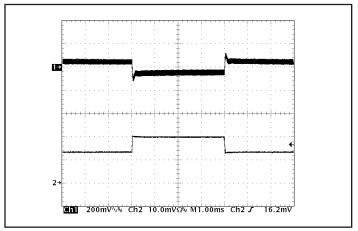
Figure 12: Output voltage response to step-change in load current (50%-75%-50% of lout(max): dI/dt = 1 A/ $\mu$ s). Load cap: 470  $\mu$ F, 30  $m\Omega$  ESR tantalum cap and 1  $\mu$ F ceramic cap. Ch 1: Vout (200 mV/div), Ch 2: lout (10 A/div).
