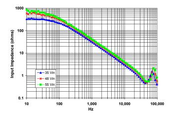
Figure 22: Magnitude of incremental input impedance (Zin = Vin/lin) for minimum, nominal, and maximum input voltage at full rated power.
