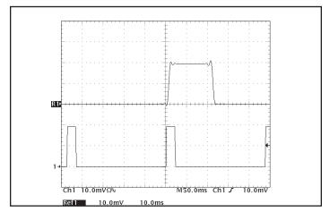
Figure 18: Load current (50 A/div) as a function of time when the converter attempts to turn on into a 1 m $\Omega$  short circuit. Top trace (10 ms/div) is an expansion of the on-time portion of the bottom trace.
