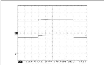
Figure 17: Output voltage response to step-change in input voltage (48 V to 55 V), at rated load current. Load cap: 15  $\mu$ F tantalum capacitor and 1  $\mu$ F ceramic cap. Ch 1: Vout (5 V/div), Ch 2: Vin (20 V/div).
