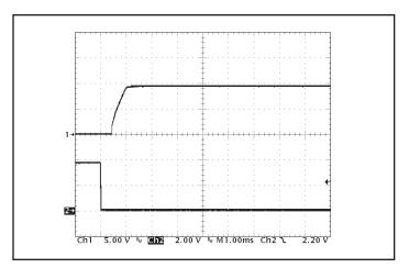
Figure 10: Turn-on transient at nominal input voltage and zero load (1 ms/div). Load cap: 3 mF output capacitance. Ch 1: Vout (5 V/div), Ch 2: ON/OFF input (2 V/div).
