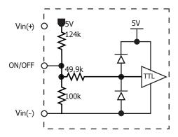
Figure B: Internal ON/OFF pin circuitry
