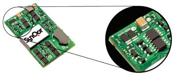
Figure G: Location of Sense Resistor
