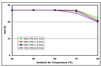
Figure 7: Maximum output power derating curves vs. ambient air temperature for airflow rates of 100 LFM through 400 LFM with air flowing across the converter from output to input (Vin = 48 V).
