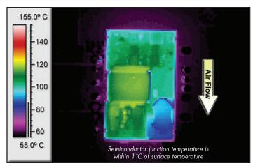
Figure 8: Thermal plot of converter at 27 A load current (240 W) with 55 °C air flowing at the rate of 200 LFM. Air is flowing across the converter from output to input (Vin = 48 V).
