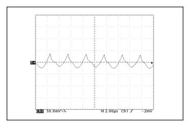
Figure 16: Output voltage ripple at nominal input voltage and full rated current (50 mV/div). Load capacitance: 1  $\mu$ F ceramic capacitor and 15  $\mu$ F tantalum capacitor. Bandwidth: 20 MHz. See Figure 13.
