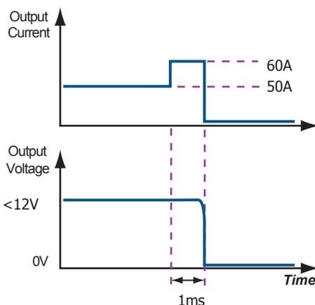
Figure C: Output Overload protection diagram (not to scale)
