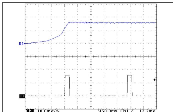
Figure 18: Load current ( $50 \text{ A/div}$ ) as a function of time when the converter attempts to turn on into a  $1 \text{ m-ohm}$  short circuit. Top trace ( $2 \text{ ms/div}$ ) is an expansion of the on-time portion of the bottom trace.
