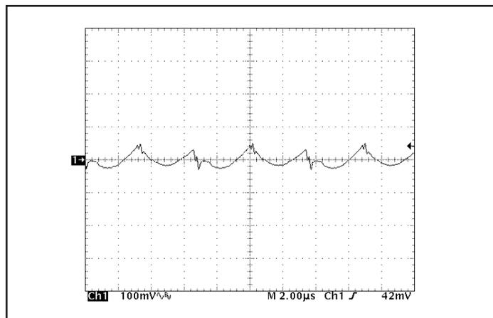
Figure 16: Output voltage ripple at nominal input voltage and rated load current ( $100 \text{ mV/div}$ ). Load capacitance:  $1 \mu\text{F}$  ceramic capacitor and  $15 \mu\text{F}$  tantalum capacitor. Bandwidth:  $20 \text{ MHz}$ . See Figure 13.
