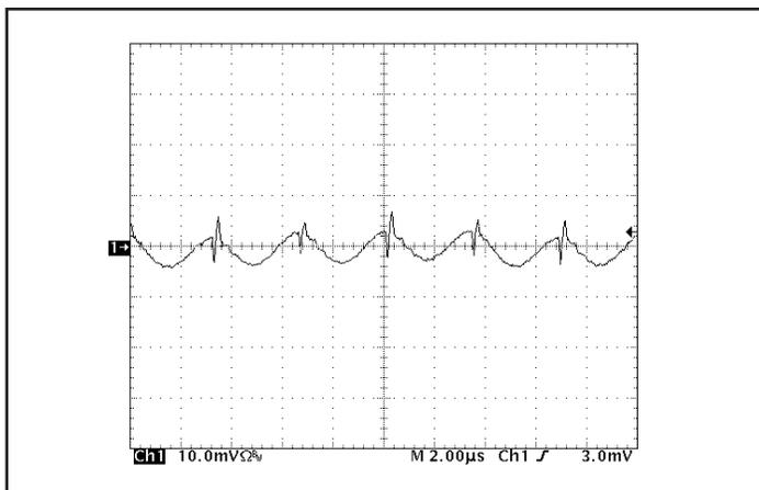
Figure 15: Input reflected ripple current,  $i_s$ , through a  $10 \mu\text{H}$  source inductor, using a  $47 \mu\text{F}$  electrolytic input capacitor ( $50 \text{ mA/div}$ ). See Figure 13.
