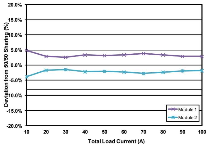
Figure I: Current share performance of 2 paralleled modules
