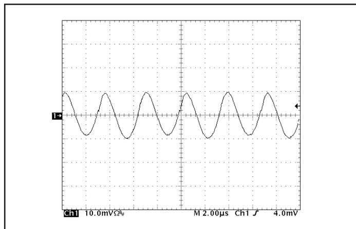
Figure 14: Input Terminal Ripple Current,  $i_c$ , at full rated output current and nominal input voltage with  $10 \mu\text{H}$  source impedance and  $47 \mu\text{F}$  electrolytic capacitor ( $500 \text{ mA/div}$ ). See Figure 13.
