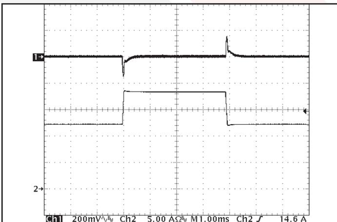
Figure 5: Output voltage response to step-change in load current (50%-75%-50% of I<sub>out</sub>(max); di/dt = 0.1A/μs). Load cap: 15μF tantalum cap and 1μF ceramic cap. Ch 1: V<sub>out</sub>, Ch 2: I<sub>out</sub>.
