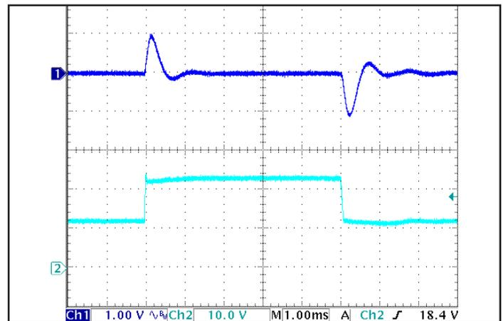
Figure 6: Output voltage response to step-change in input voltage (250 V/ms). Load cap: 100 μF electrolytic output capacitance. Ch 1: V<sub>out</sub> (1 V/div), Ch 2: V<sub>in</sub> (10 V/div).
