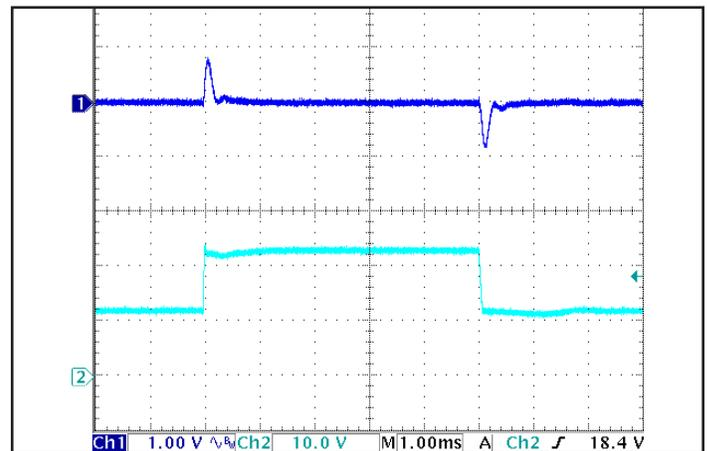
Figure 6: Output voltage response to step-change in input voltage (250V/ms). Load cap: 100 $\mu\text{F}$  electrolytic output capacitance. Ch 1:  $V_{out}$  (1V/div), Ch 2:  $V_{in}$  (10V/div).
