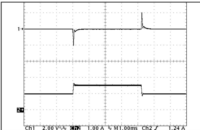
Figure 5: Output voltage response to step-change in load current (66% -100% -66% of I<sub>out</sub>(max); dI/dt = 0.02 A/μs). Load cap: 1 μF ceramic cap. Ch 1: V<sub>out</sub> (2 V/div), Ch 2: I<sub>out</sub> (1 A/div).
