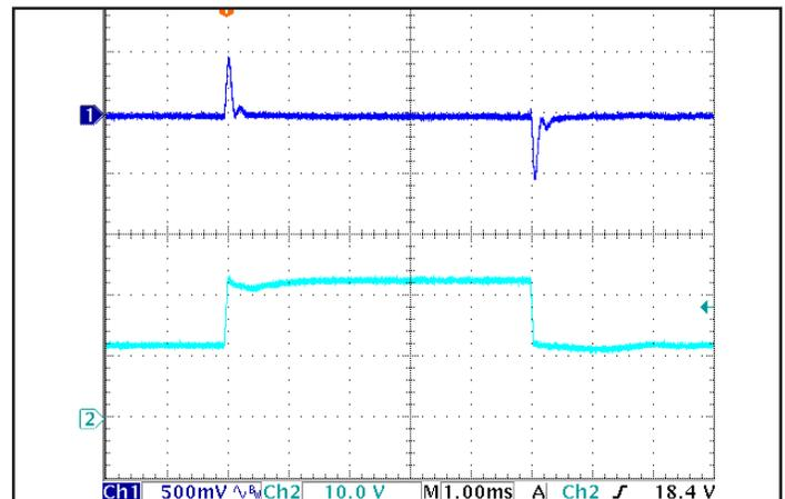
Figure 6: Output voltage response to step-change in input voltage (250 V/ms). Load cap: 100 μF electrolytic output capacitance. Ch 1: V<sub>out</sub> (500 mV/div), Ch 2: V<sub>in</sub> (10 V/div).
