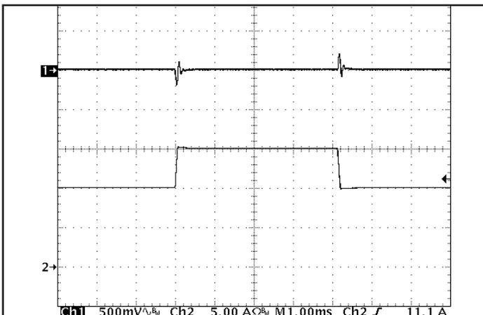
Figure 5: Output voltage response to step-change in load current (66% -100% -66% of  $I_{out(max)}$ ;  $dI/dt = 0.1 A/\mu s$ ). Load cap: 15  $\mu F$  tantalum cap and 1  $\mu F$  ceramic cap. Ch 1:  $V_{out}$  (500 mV/div), Ch 2:  $I_{out}$  (5 A/div).
