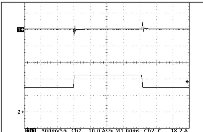
Figure 5: Output voltage response to step-change in load current (66% -100% -66% of I<sub>out</sub>(max); dI/dt = 0.2 A/μs). Load cap: 15 μF tantalum cap and 1 μF ceramic cap. Ch 1: V<sub>out</sub> (500 mV/div), Ch 2: I<sub>out</sub> (10 A/div).
