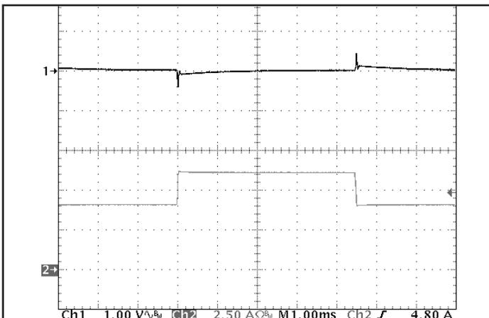
Figure 5: Output voltage response to step-change in load current (66% -100% -66% of I<sub>out</sub>(max); dI/dt = 0.1 A/μs). Load cap: 15 μF tantalum cap and 1 μF ceramic cap. Ch 1: V<sub>out</sub> (1 V/div), Ch 2: I<sub>out</sub> (2.5 A/div).
