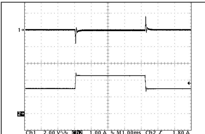
Figure 5: Output voltage response to step-change in load current (66% -100% -66% of I<sub>out</sub>(max); dI/dt = 0.05 A/μs). Load cap: 1 μF ceramic cap. Ch 1: V<sub>out</sub> (2 V/div), Ch 2: I<sub>out</sub> (1 A/div).
