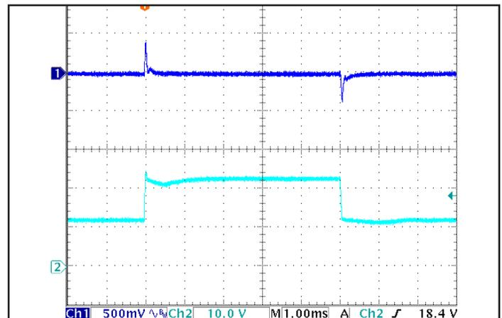
Figure 6: Output voltage response to step-change in input voltage (250 V/ms). Load cap: 100  $\mu F$  electrolytic output capacitance. Ch 1:  $V_{out}$  (500 mV/div), Ch 2:  $V_{in}$  (10 V/div).
