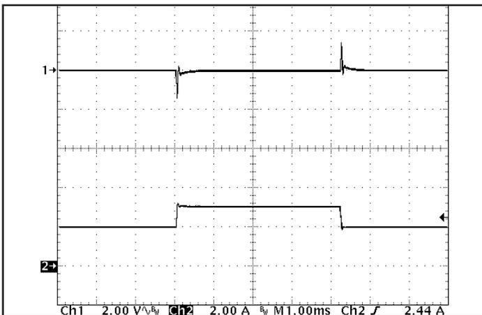
Figure 5: Output voltage response to step-change in load current (66% -100% -66% of  $I_{out(max)}$ ;  $dI/dt = 0.08 \text{ A}/\mu\text{s}$ ). Load cap: 1  $\mu\text{F}$  ceramic cap. Ch 1:  $V_{out}$  (2 V/div), Ch 2:  $I_{out}$  (2 A/div).
