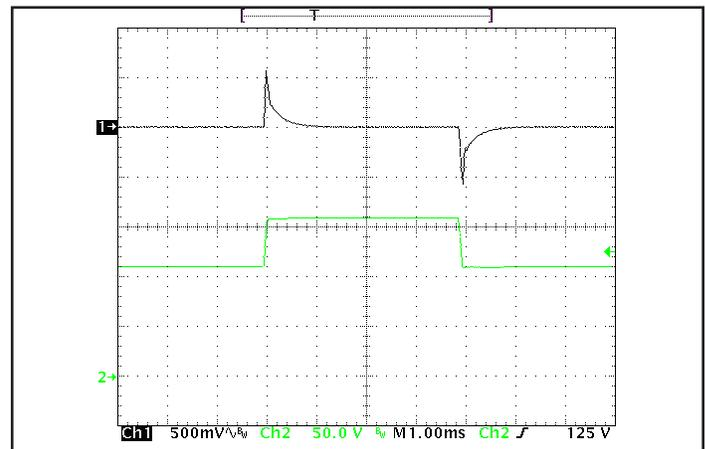
Figure 6: Output voltage response to step-change in input voltage (1000 V/ms), at Max. load current. Load cap: 1 μF ceramic cap. Ch 1: V<sub>out</sub>, Ch 2: V<sub>in</sub>.
