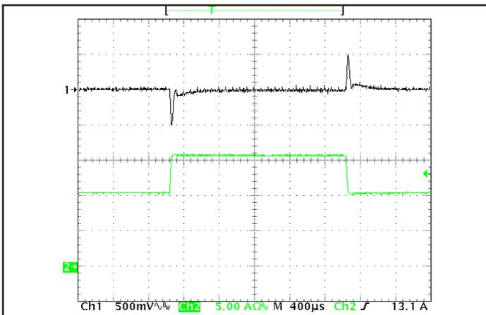
Figure 5: Output voltage response to step-change in load current (65% -100% -65% of I<sub>out</sub>(max); dI/dt = 0.1 A/μs. Load cap: 15 μF tantalum cap and 1 μF ceramic cap. Ch 1: V<sub>out</sub>, Ch 2: I<sub>out</sub> (5 A/div).
