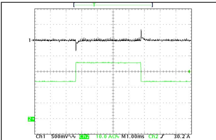
Figure 5: Output voltage response to step-change in load current (65% -100% -65% of  $I_{out(max)}$ ;  $dI/dt = 0.1 A/\mu s$ . Load cap: 15  $\mu F$  tantalum cap and 1  $\mu F$  ceramic cap. Ch 1:  $V_{out}$ , Ch 2:  $I_{out}$  (10 A/div).
