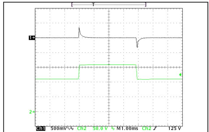
Figure 6: Output voltage response to step-change in input voltage (1000 V/ms), at Max. load current. Load cap: 15 μF tantalum cap and 1 μF ceramic cap. Ch 1: V<sub>out</sub>, Ch 2: V<sub>in</sub>.
