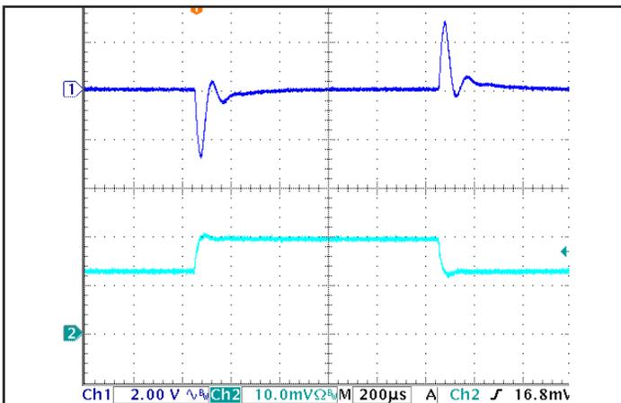
Figure 5: Output voltage response to step-change in load current (65% -100% -65% of I<sub>out</sub>(max); dI/dt = 0.1 A/μs. Load cap: 1 μF ceramic cap. Ch 1: V<sub>out</sub>, Ch 2: I<sub>out</sub> (2 A/div).
