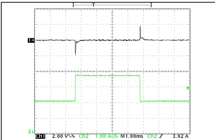
Figure 5: Output voltage response to step-change in load current (65% -100% -65% of I<sub>out</sub>(max); dI/dt = 0.1 A/μs. Load cap: 1 μF ceramic cap. Ch 1: V<sub>out</sub>, Ch 2: I<sub>out</sub> (1 A/div).
