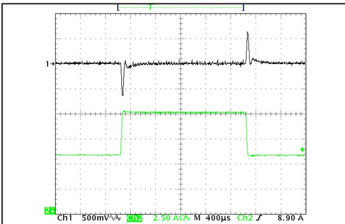
Figure 5: Output voltage response to step-change in load current (65% -100% -65% of I<sub>out</sub>(max); dI/dt = 0.1 A/μs. Load cap: 15 μF tantalum cap and 1 μF ceramic cap. Ch 1: V<sub>out</sub>, Ch 2: I<sub>out</sub> (2.5 A/div).
