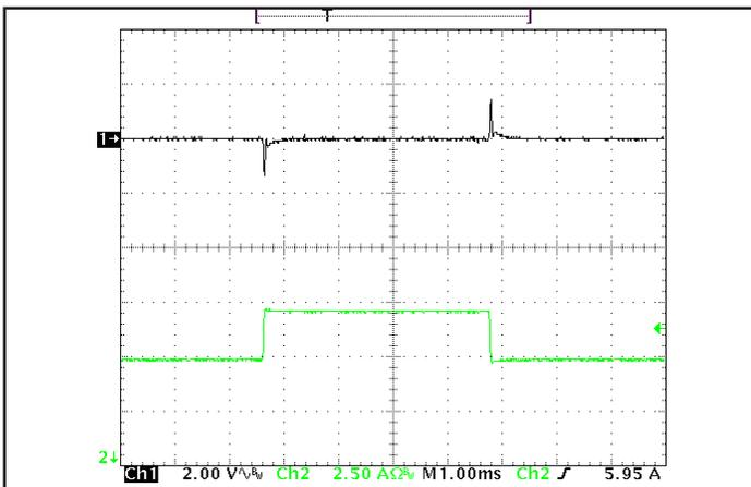
Figure 5: Output voltage response to step-change in load current (65% -100% -65% of I<sub>out</sub>(max); dI/dt = 0.1 A/μs. Load cap: 1 μF ceramic cap. Ch 1: V<sub>out</sub>, Ch 2: I<sub>out</sub> (2.5 A/div).
