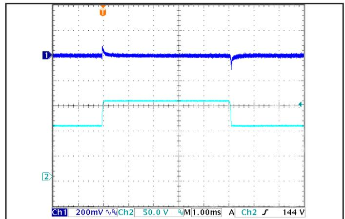
Figure 6: Output voltage response to step-change in input voltage (1000 V/ms). Load cap: 100 μF, electrolytic output capacitance. Ch 1: V<sub>out</sub> (200 mV/div), Ch 2: V<sub>in</sub> (50 V/div).
