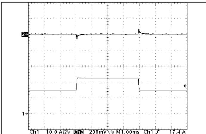
Figure 5: Output voltage response to step-change in load current (66%-100%-%66% of I<sub>out</sub>(max); dI/dt = 0.1 A/μs). Load cap: 15 μF tantalum cap and 1 μF ceramic cap. Ch 1: I<sub>out</sub> (10 A/div), Ch 2: V<sub>out</sub> (200 mV/div).
