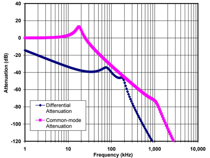
**Figure 1:** Simulation of calculated common-mode and differential-mode current attenuation. The plots show the ratio of the measured current in a 50Ω LISN sensing port connected to pins 1 or 3 to the noise current injected into pins 4 and 6. See Figs. 2 & 3.
