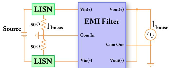
**Figure 3:** Common-Mode Current Attenuation,  $I_{meas} / I_{noise}$
