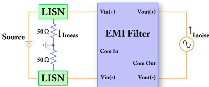
**Figure 2:** Differential-Mode Current Attenuation,  $I_{meas} / I_{noise}$
