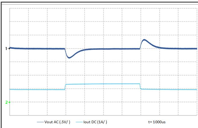
Figure 5: Output voltage response to step-change in load current (50% -75% -50% of I<sub>out</sub>(max); dI/dt = 0.1 A/μs). Load cap: 100 μF electrolytic cap and 1 μF ceramic cap. Ch 1: V<sub>out</sub> (500 mV/div), Ch 2: I<sub>out</sub> (1 A/div).
