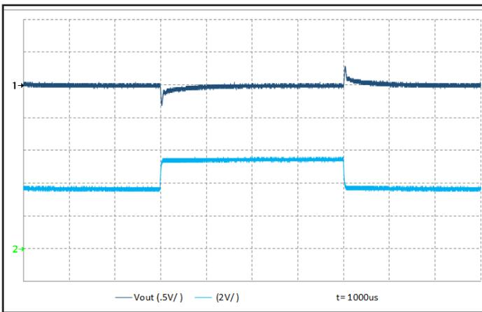
Figure 5: Output voltage response to step-change in load current (50% - 75% - 50% of I<sub>out</sub>(max); dI/dt = 0.1 A/μs). Load cap: 100 μF electrolytic cap and 1 μF ceramic cap. Ch 1: V<sub>out</sub> (500 mV/div), Ch 2: I<sub>out</sub> (2 A/div).
