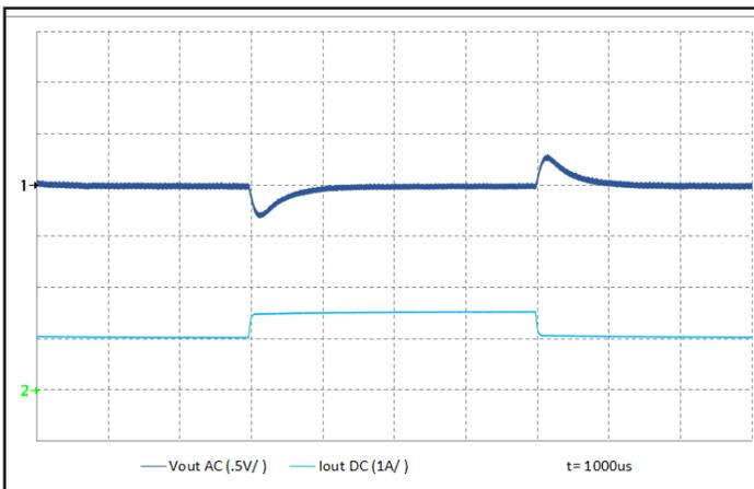
Figure 5: Output voltage response to step-change in load current (50% -75% -50% of  $I_{out}(max)$ ;  $dI/dt = 0.1 A/\mu s$ ). Load cap: 100  $\mu F$  electrolytic cap and 1  $\mu F$  ceramic cap. Ch 1:  $V_{out}$  (500 mV/div), Ch 2:  $I_{out}$  (1 A/div).
