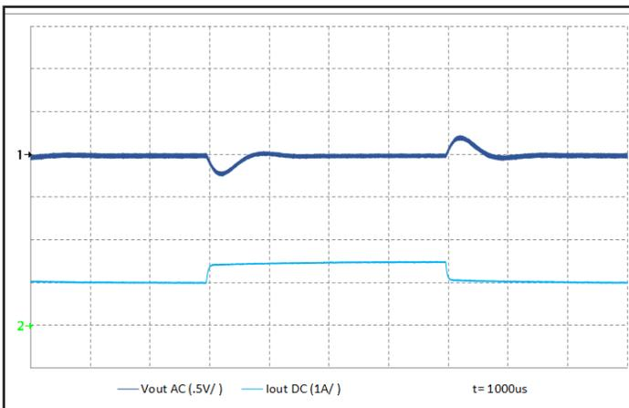
Figure 5: Output voltage response to step-change in load current (50% -75% -50% of I<sub>out</sub>(max); dI/dt = 0.1 A/μs). Load cap: 100 μF electrolytic cap and 1 μF ceramic cap. Ch 1: V<sub>out</sub> (500 mV/div), Ch 2: I<sub>out</sub> (500 mA/div).
