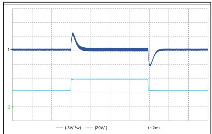
Figure 6: Output voltage response to step-change in input voltage (250 V/ms). Load cap: 100 μF, electrolytic output capacitance. Ch 1: V<sub>out</sub> (500 mV/div), Ch 2: V<sub>in</sub> (20 V/div).
