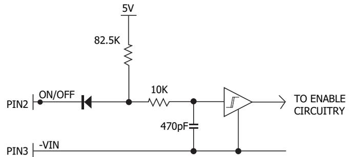
Figure B: Internal ON/OFF pin circuitry
