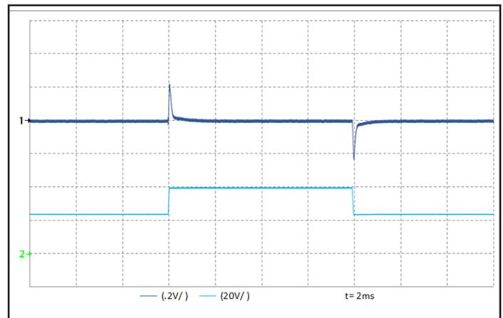
Figure 6: Output voltage response to step-change in input voltage (250 V/ms). Load cap: 100 μF, electrolytic output capacitance. Ch 1: V<sub>out</sub> (200 mV/div), Ch 2: V<sub>in</sub> (20 V/div).
