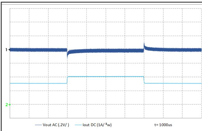
Figure 5: Output voltage response to step-change in load current (50% -75% -50% of I<sub>out</sub>(max); dI/dt = 0.1 A/μs). Load cap: 100 μF electrolytic cap and 1 μF ceramic cap. Ch 1: V<sub>out</sub> (200 mV/div), Ch 2: I<sub>out</sub> (5 A/div).
