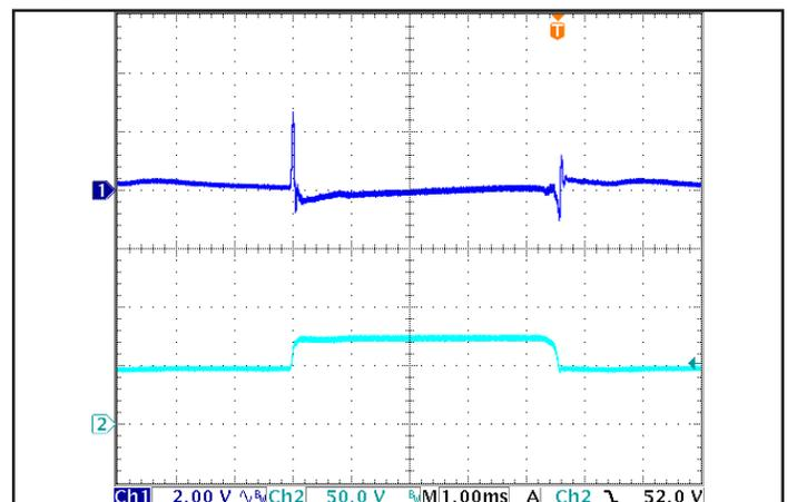
Figure 6: Output Voltage Response to Step-Change in Input Voltage (500 V/ms), at Max. load current. Load cap: 100 μF electrolytic cap and 1 μF ceramic cap. Ch 1: V<sub>out</sub>, Ch 2: V<sub>in</sub>.
