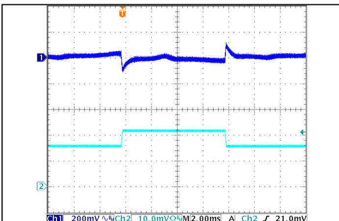
Figure 5: Output Voltage Response to Step-Change in Load Current (50 %- 50 % of Iout(max); dI/dt = 0.1 A/μs). Load cap: 15 μF tantalum cap and 1 μF ceramic cap. Ch 1: Vout, Ch 2: Iout (20 A/div).
