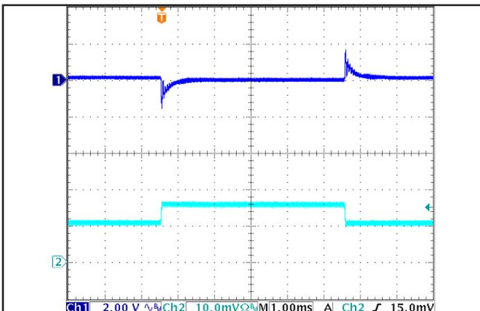
Figure 5: Output Voltage Response to Step-Change in Load Current (50% -75% -50% of Iout(max)); dl/dt = 0.1 A/μs. Load cap: 1 μF ceramic cap. Ch 1: Vout, Ch 2: Iout (5 A/div).
