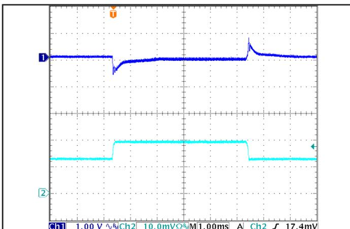
Figure 5: Output Voltage Response to Step-Change in Load Current (50% -75% -50% of  $I_{out(max)}$ ;  $dl/dt = 0.1 A/\mu s$ . Load cap: 15  $\mu F$  tantalum cap and 1  $\mu F$  ceramic cap. Ch 1:  $V_{out}$ , Ch 2:  $I_{out}$  (10 A/div).
