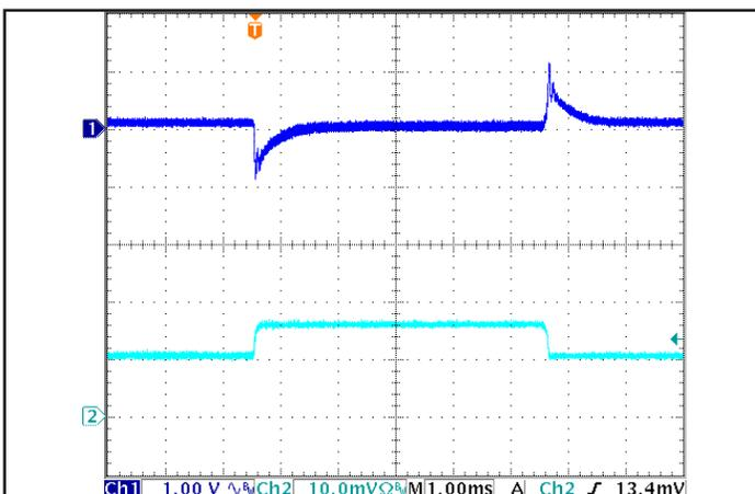
Figure 5: Output Voltage Response to Step-Change in Load Current (50% -75% -50% of I<sub>out</sub>(max); dI/dt = 0.1 A/μs. Load cap: 15 μF tantalum cap and 1 μF ceramic cap. Ch 1: V<sub>out</sub>, Ch 2: I<sub>out</sub> (10 A/div).
