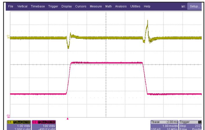
Figure 6: Output voltage response to step-change in input voltage (180V - 425V - 180V), at 6.25A load current. Load cap: 15µF tantalum capacitor and 1µF ceramic cap. Ch 1: V<sub>out</sub> (1V/div), Ch 2: V<sub>in</sub> (100V/div).
