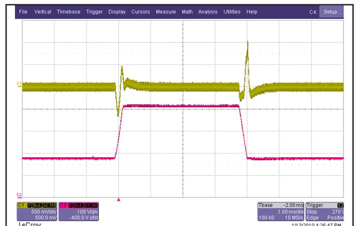
Figure 6: Output voltage response to step-change in input voltage (180V - 425V - 180V), at 10.7A load current. Load cap: 15μF tantalum capacitor and 1μF ceramic cap. Ch 1: V<sub>out</sub> (500mV/div), Ch 2: V<sub>in</sub> (100V/div).
