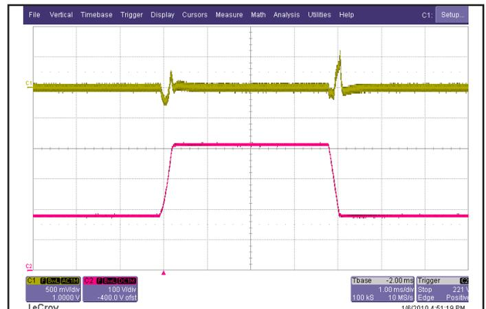
Figure 6: Output voltage response to step-change in input voltage (180V - 425V - 180V), at 20A load current. Load cap: 15μF tantalum capacitor and 1μF ceramic cap. Ch 1: V<sub>out</sub> (500mV/div), Ch 2: V<sub>in</sub> (100V/div).
