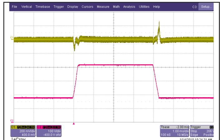
Figure 6: Output voltage response to step-change in input voltage (180V - 425V - 180V), at 50A load current. Load cap: 15μF tantalum capacitor and 1μF ceramic cap. Ch 1: V<sub>out</sub> (200mV/div), Ch 2: V<sub>in</sub> (100V/div).
