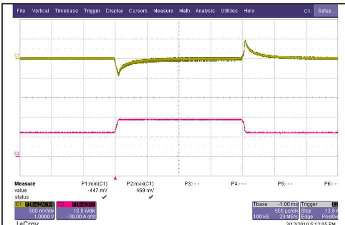
Figure 5: Output voltage response to step-change in load current (50%-75%-50% of I<sub>out</sub>(max); dI/dt = 0.1A/μs). Load cap: 15μF tantalum cap and 1μF ceramic cap. Ch 1: V<sub>out</sub> (500mV/div), Ch 2: I<sub>out</sub> (10A/div).
