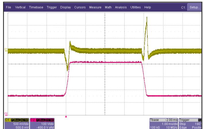
Figure 6: Output voltage response to step-change in input voltage (180V - 425V - 180V), at 6.25A load current. Load cap: 15μF tantalum capacitor and 1μF ceramic cap. Ch 1: V<sub>out</sub> (1V/div), Ch 2: V<sub>in</sub> (100V/div).
