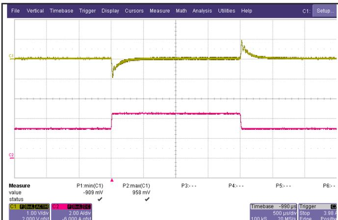
Figure 5: Output voltage response to step-change in load current (50%-75%-50% of I<sub>out</sub>(max); dI/dt = 0.1A/µs). Load cap: 15µF tantalum cap and 1µF ceramic cap. Ch 1: V<sub>out</sub> (1V/div), Ch 2: I<sub>out</sub> (2A/div).
