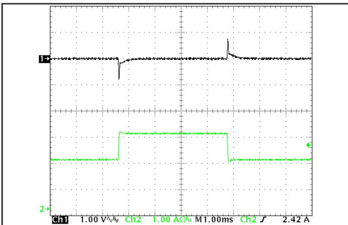
Figure 5: Output response to load current step for QTC version of product (50% -75% -50% of Iout(max); dI/dt = 0.2 A/μs). Load cap: 1 μF ceramic capacitor. Ch 1: Vout, Ch 2: Iout.
