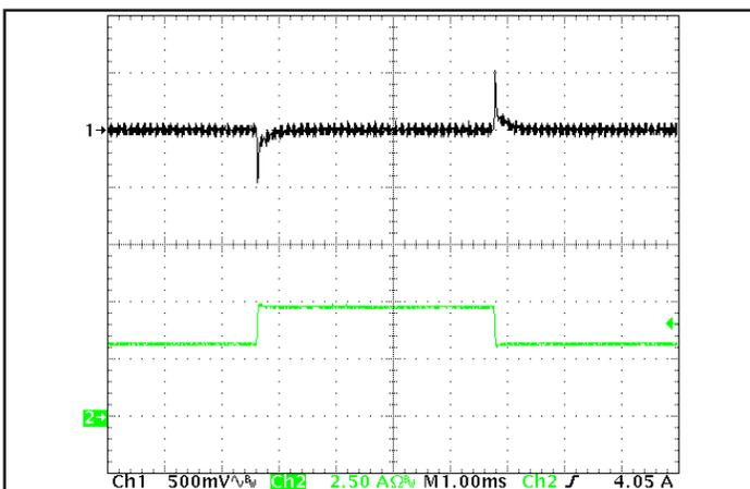
Figure 5: Output response to load current step for QTC version of product (50% -75% -50% of Iout(max); dI/dt = 0.2 A/μs). Load cap: 1 μF ceramic and 15 μF tantalum capacitors. Ch 1: Vout, Ch 2: Iout.
