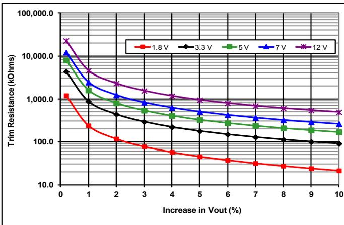
Common Figure 3: Trim-Up Graph for 1.8 to 12V outputs.
