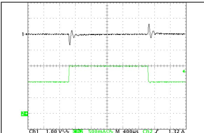
Figure 5: Output voltage response to step-change in load current (50 % -75 % -50 % of I<sub>out</sub>(max); dI/dt = 0.05 A/μs). Load cap: 1 μF ceramic cap. Ch 1: V<sub>out</sub>, Ch 2: I<sub>out</sub>.
