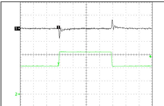
Figure 5: Output voltage response to step-change in load current (50% -75% -50% of I<sub>out</sub>(max); dI/dt = 0.05 A/μs). Load cap: 15 μF tantalum cap and 1 μF ceramic cap. Ch 1: V<sub>out</sub>, Ch 2: I<sub>out</sub>.
