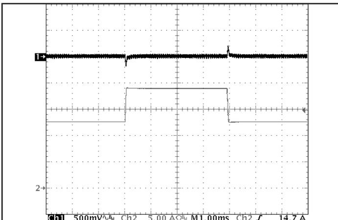
Figure 5: Output voltage response to step-change in load current (50% -75% -50% of I<sub>out</sub>(max); dI/dt = 0.2 A/μs). Load cap: 1 μF ceramic and 15 μF tantalum capacitors. Ch 1: V<sub>out</sub>, Ch 2: I<sub>out</sub>. Timescale: 1.00ms/div.
