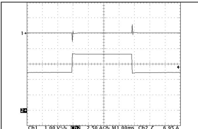
Figure 5: Output voltage response to step-change in load current (50% -75% -50% of Iout(max); dI/dt = 0.2 A/μs). Load cap: 1 μF ceramic and 15 μF tantalum capacitors. Ch 1: Vout, Ch 2: Iout. Timescale: 1.00ms/div.
