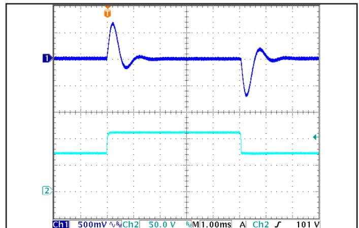
Figure 6: Output voltage response to step-change in input voltage (1000 V/ms). Load cap: 1  $\mu F$  ceramic capacitor. Ch 1:  $V_{out}$ , Ch 2:  $V_{in}$ . Timescale: 1.00ms/div.
