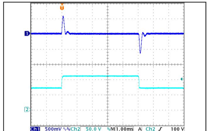
Figure 6: Output voltage response to step-change in input voltage (1000 V/ms). Load cap: 1 μF ceramic capacitor. Ch 1: V<sub>out</sub>, Ch 2: V<sub>in</sub>. Timescale: 1.00ms/div.
