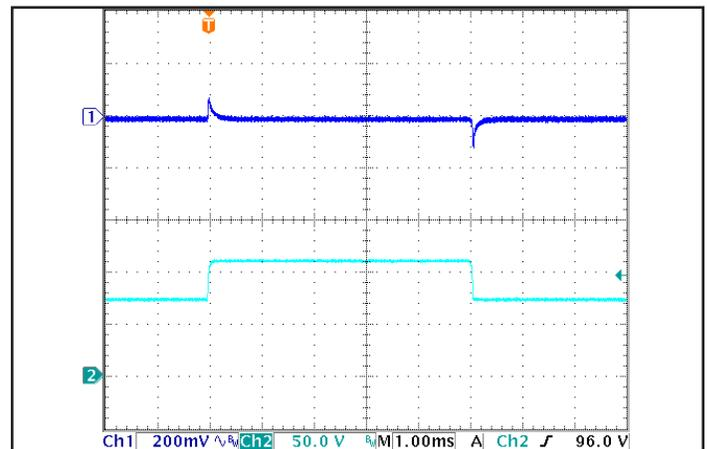
Figure 6: Output voltage response to step-change in input voltage (1000 V/ms). Load cap: 1 μF ceramic and 15 μF tantalum capacitors. Ch 1: V<sub>out</sub>, Ch 2: V<sub>in</sub>. Timescale: 1.00ms/div.
