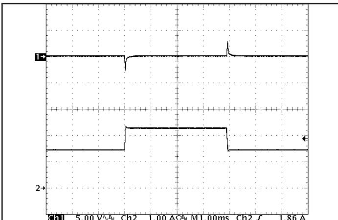
Figure 5: Output voltage response to step-change in load current (50% -75% -50% of  $I_{out(max)}$ ;  $dI/dt = 0.2 A/\mu s$ ). Load cap: 1  $\mu F$  ceramic capacitor. Ch 1:  $V_{out}$ , Ch 2:  $I_{out}$ . Timescale: 1.00ms/div.
