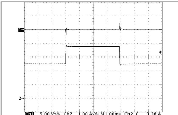
Figure 5: Output voltage response to step-change in load current (50% -75% -50% of I<sub>out</sub>(max); dI/dt = 0.2 A/μs). Load cap: 1 μF ceramic capacitor. Ch 1: V<sub>out</sub>, Ch 2: I<sub>out</sub>. Timescale: 1.00ms/div.
