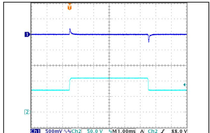
Figure 6: Output voltage response to step-change in input voltage (1000 V/ms). Load cap: 1 μF ceramic and 15 μF tantalum capacitors. Ch 1: Vout, Ch 2: Vin. Timescale: 1.00ms/div.
