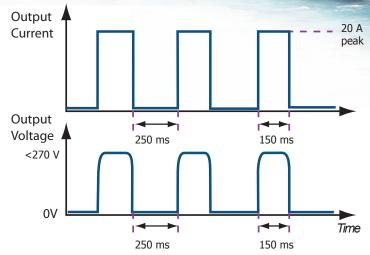
Figure E: Output Short Circuit and Auto-Resetting protection diagram (not to scale)
