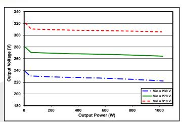
Figure 7: Output voltage vs. output power, regulation curves for minimum, nominal, and maximum input voltage at TCASE=25 °C.
