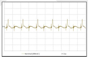
Figure 15: Input terminal ripple, ic, at full load and nominal voltage with 10 µH source impedance and 100µF electrolytic capacitor(200 mA/div), Bandwidth: Full. Timescale: 2 µs/div. See Figure 12.
