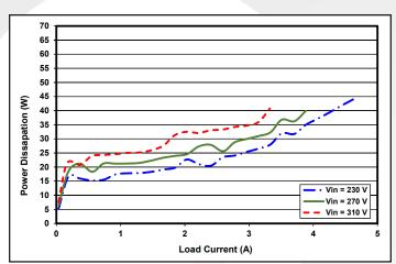
Figure 3: Power dissipation vs. load current for minimum, nominal, and maximum input voltage at TCASE=25 °C.
