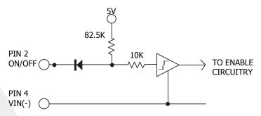
Figure B: Internal ON/OFF pin circuitry
