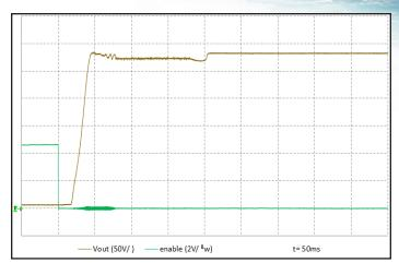
Figure 8: Turn-on transient at no load and zero output capacitance initiated by ENA. Input voltage pre-applied. Ch 1: Vout (50 V/div). Ch 2: ENA (2 V/div). Timescale: 50 ms/div.
