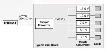
Figure A: Example of Intermediate Bus Architecture using isolated or nonisolated converters.
