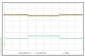
Figure 13: Output voltage response to step-change in load current 50%-75%-50% of lout (max). Zero output capacitance. Ch1: Vout (10 V/div). Ch 2: Iout (2 A/div). Timescale: 10 ms/div. Plot created using measured Vout minus Vin/Turns Ratio.
