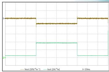
Figure 14: Output voltage response to step-change in load current 10%-100%-10% of lout (max). Zero output capacitance. Ch1: Vout (10 V/div). Ch 2: Iout (2 A/div). Timescale: 10 ms/div. Plot created using measured Vout minus Vin/Turns Ratio.
