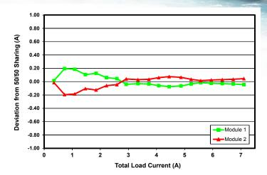
Figure I: Typical current share performance of 2 paralleled modules
