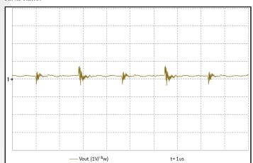
Figure 16: Output voltage ripple, Vout, at nominal input voltage and full load (1 V/div), Measured with 1.1uF capacitance across the output terminals. Bandwidth: 20 MHz. Timescale: 1 µs/div. See Figure 12.
