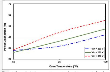
Figure 4: Power dissipation vs. case temperature for minimum, nominal, and maximum input voltage and 100% rated power.
