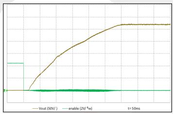
Figure 9: Turn-on transient at half resistive load and 47 uF output capacitance initiated by ENA. Input voltage pre-applied. Ch 1: Vout (50 V/div). Ch 2: ENA (2 V/div). Timescale: 50 ms/div.
