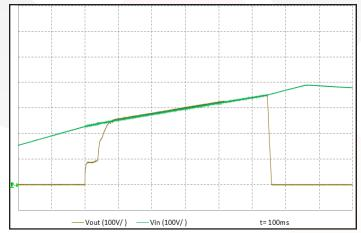
Figure 11: Turn-on and Turn-off behavior as a function of Vin. ENA previously enabled. Ch 1: Vout (100 V/div). Ch 2: Vin (100 V/div). Timescale: 100 ms/div.
