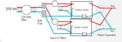
Figure H: Recommended physical implementation of two Bus Oor's in parallel.
