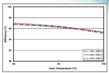
Figure 2: Efficiency vs. case temperature for minimum, nominal, and maximum input voltage and 100% rated power.
