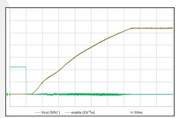
Figure 10: Turn-on transient at half resistive load and 400 uF output capacitance initiated by ENA. Input voltage pre-applied. Ch 1: Vout (50 V/div). Ch 2: ENA (2 V/div). Timescale: 50 ms/div.
