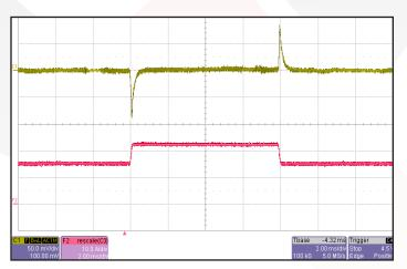
Figure 11: Output voltage response to step-change in load current (50%-75%-50% of lout(max);  $dI/dt=0.1~A/\mu s$ ). Load cap:  $1~\mu F$  ceramic and 15  $\mu F$  tantalum capacitors. Ch 1: Vout (50mV/div), Ch 2: lout (10A/div).
