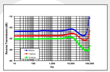
Figure 15: Magnitude of incremental reverse transmission (RT = iin/lout) for minimum, nominal, and maximum input voltage at full rated power.
