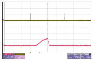
**Figure 18:** Load current (50A/div) as a function of time (0.5ms/div and 50ms/div) when the converter attempts to turn on into a 10 m $\Omega$  short circuit.
