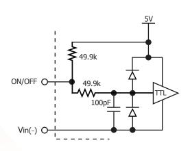
Figure B: Internal ON/OFF pin circuitry
