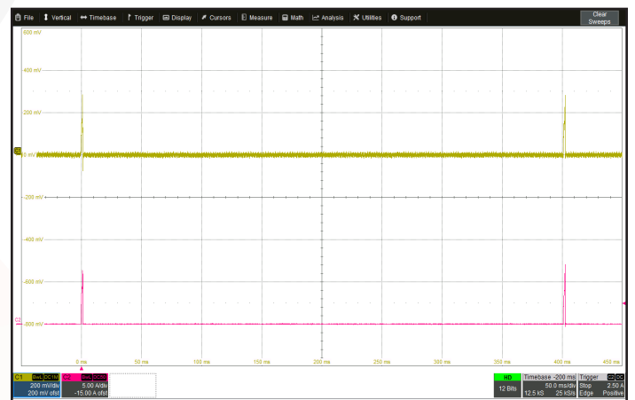
Figure 18: A short circuit across the output terminals. Ch 1: V_{out} (200 mV/div). Ch 2: I_{out} (5 A/div). Timescale: 50ms/div.
