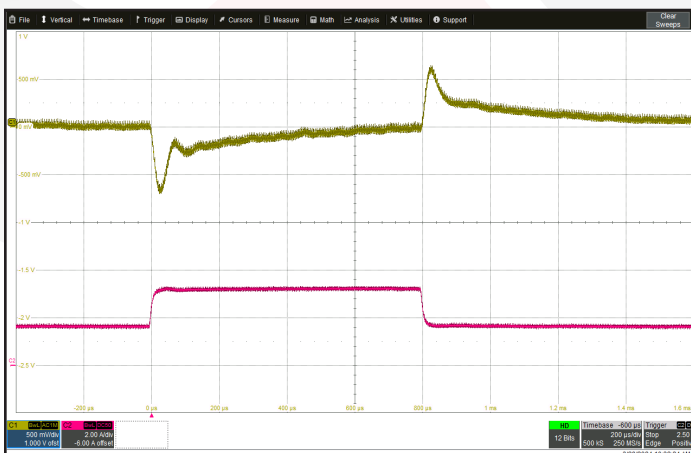
Figure 11: Output voltage response to step-change in load current 50%-100%-50% of Iout (max). No external load capacitance. Ch 1: Vout (500 mV/div). Ch 2: Iout (2 A/div). Timescale: 200µs/div.
