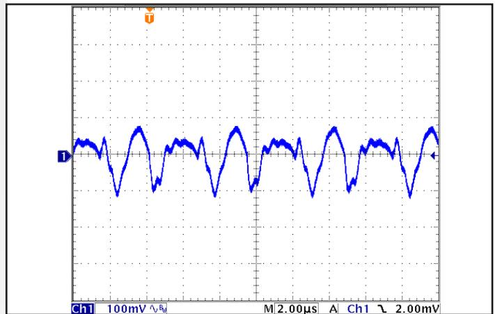
**Figure 10:** Output voltage ripple, Vout, at nominal input voltage and rated load current (100 mV/div). Load capacitance: 10  $\mu$ F tantalum capacitor. Bandwidth: 20 MHz. See Figure 17. Horizontal Scale: 2  $\mu$ s/div
