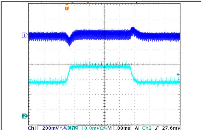
**Figure 11:** Output voltage response to step-change in load current (50%-75%-50% of Iout(max);  $di/dt = 0.1 A/\mu s$ ). Load cap: 1  $\mu$ F ceramic and 15  $\mu$ F tantalum capacitors. Ch 1: Vout (200 mV/div), Ch 2: Iout (20 A/div). Horizontal Scale: 1 ms/div
