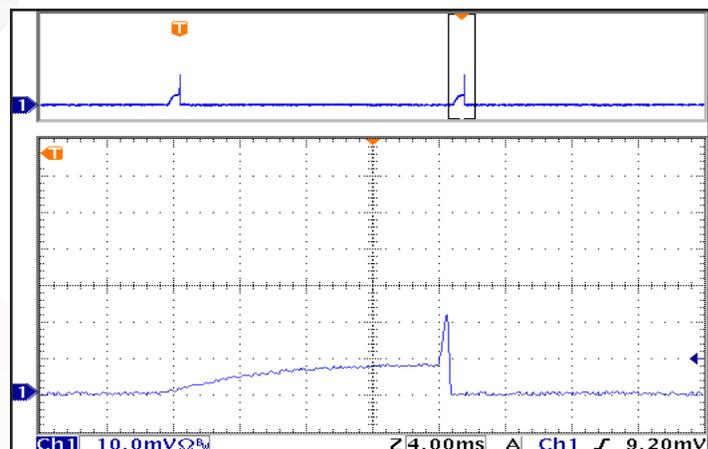
Figure 18: Load current (50 A/div) as a function of time (4 ms/div and 100 ms/div) when the converter attempts to turn on into a 10 m Ohm short circuit.
