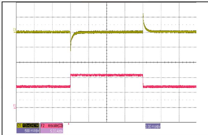
Figure 11: Output voltage response to step-change in load current (50%-75%-50% of  $I_{out(max)}$ ;  $dI/dt = 0.1\text{ A}/\mu\text{s}$ ). Load cap:  $1\mu\text{F}$  ceramic and  $15\mu\text{F}$  tantalum capacitors. Ch 1:  $V_{out}$  (500mV/div), Ch 2:  $I_{out}$  (5A/div).
