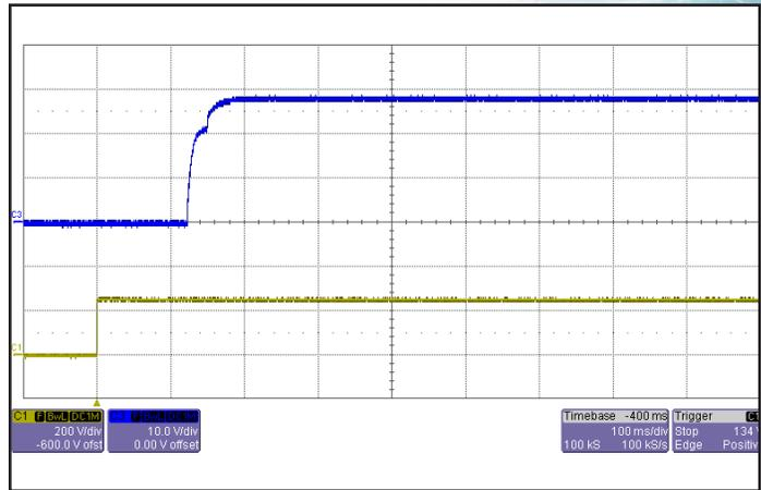
Figure 8: Turn-on transient at full resistive load and zero output capacitance initiated by Vin. ON/OFF Pin previously low. Ch 1: Vin (200V/div). Ch 3: Vout (10V/div).
