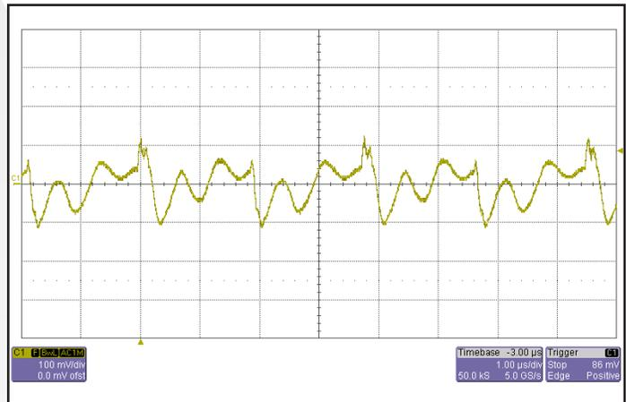
Figure 10: Output voltage ripple,  $V_{out}$ , at nominal input voltage and rated load current (100 mV/div). Load capacitance:  $1\mu\text{F}$  ceramic capacitor and  $10\mu\text{F}$  tantalum capacitor. Bandwidth: 10 MHz. See Figure 17.
