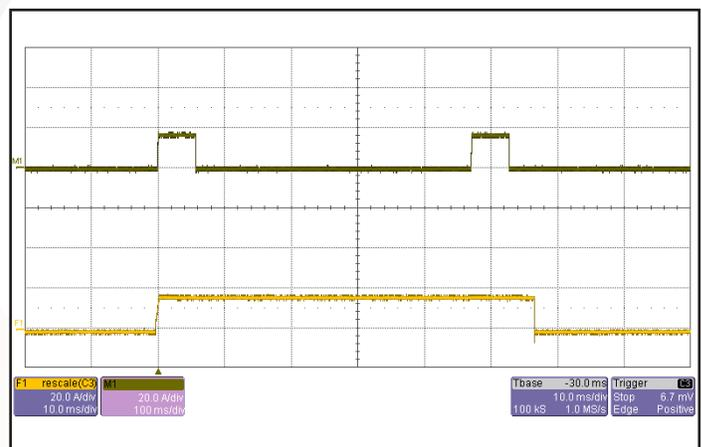
Figure 18: Load current (20A/div) as a function of time (10ms/div and 100ms/div) when the converter attempts to turn on into a 10 mΩ short circuit.
