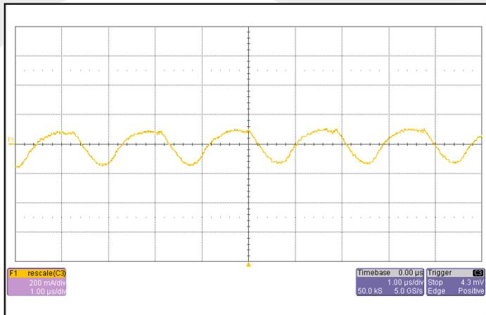
Figure 9: Input terminal current ripple,  $i_C$ , at full rated output current and nominal input voltage with  $100\mu\text{H}$  source impedance and  $47\mu\text{F}$  electrolytic Capacitor (200 mA/div). Bandwidth: 20MHz. See Figure 17.
