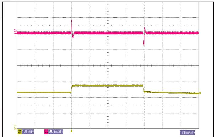
Figure 12: Output voltage response to step-change in input voltage (250V/ms). Load cap:  $100\mu\text{F}$  electrolytic output capacitance. Ch 1:  $V_{in}$  (100V/div), Ch 2:  $V_{out}$  (500mV/div).
