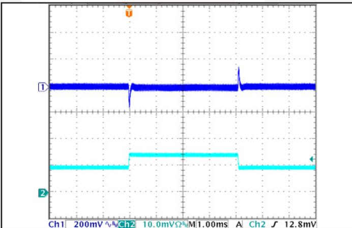
Figure 11: Output voltage response to step-change in load current (50-75-50% of  $I_{out(max)}$ ;  $di/dt = 0.1 A/\mu s$ ). Load cap: 1 µF ceramic and 100 µF electrolytic capacitors. Ch 1:  $V_{out}$  (200mV/div), Ch 2:  $I_{out}$  (5A/div). Timescale: 1.00ms/div.
