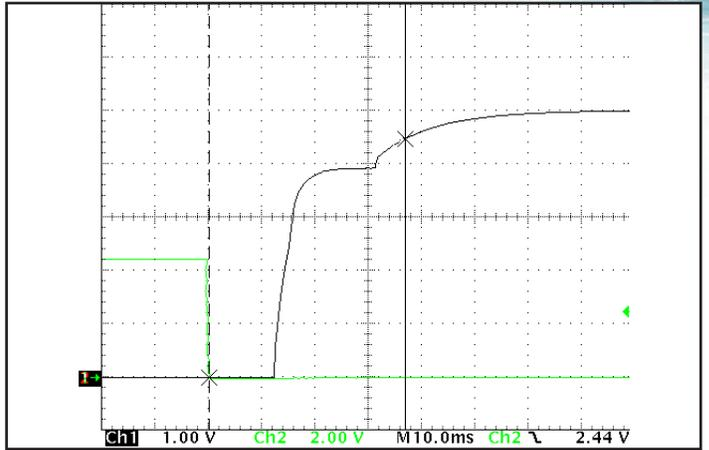
Figure 8: Typical startup waveform. Input voltage pre-applied, Ch 1:  $V_{out}$  (1V/div). Ch 2: ON/OFF Pin (2V/div). Timescale: 10.0ms/div.
