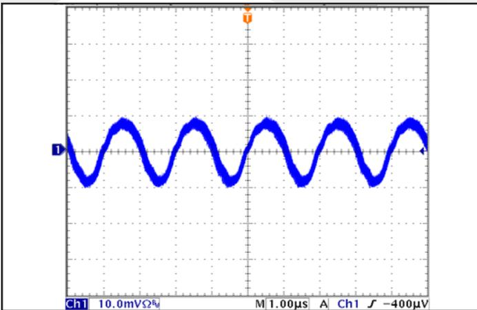
Figure 9: Input terminal current ripple,  $i_c$ , at full rated output current and nominal input voltage with SynQor MCOTS filter module (100 mA/div). Bandwidth: 20 MHz. Timescale: 1µsec/div. See Figure 17.
