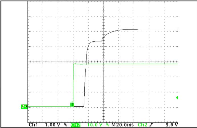
Figure 7: Turn-on transient at full load initiated by Nominal  $V_{in}$ . ON/OFF Pin previously low. Ch 1:  $V_{out}$  (1V/div). Ch 2:  $V_{in}$  (10V/div). Timescale: 20.0ms/div.
