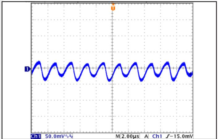
Figure 10: Output voltage ripple,  $V_{out}$ , at nominal input voltage and rated load current (50 mV/div). Load capacitance: 1µF ceramic capacitor and 15µF tantalum capacitor. Timescale: 2µsec/div. Bandwidth: 20 MHz. See Figure 17.
