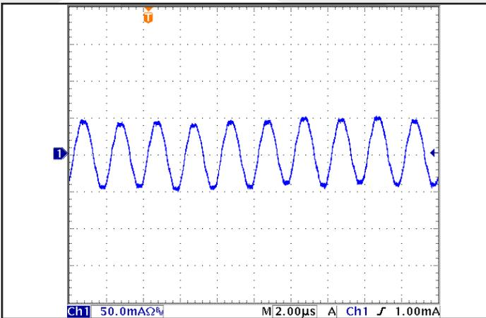
Figure 9: Input terminal current ripple,  $i_c$ , at full rated output current and nominal input voltage with SynQor MCOTS filter module (50 mA/div). Bandwidth: 20 MHz. Timescale: 2.00µs/div. See Figure 17.
