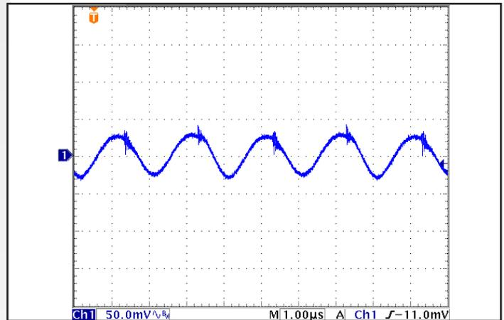
Figure 10: Output voltage ripple,  $V_{out}$ , at nominal input voltage and rated load current (50 mV/div). Load capacitance: 1µF ceramic capacitor and 15µF tantalum capacitor. Bandwidth: 20 MHz. Timescale: 1.00µs/div. See Figure 17.
