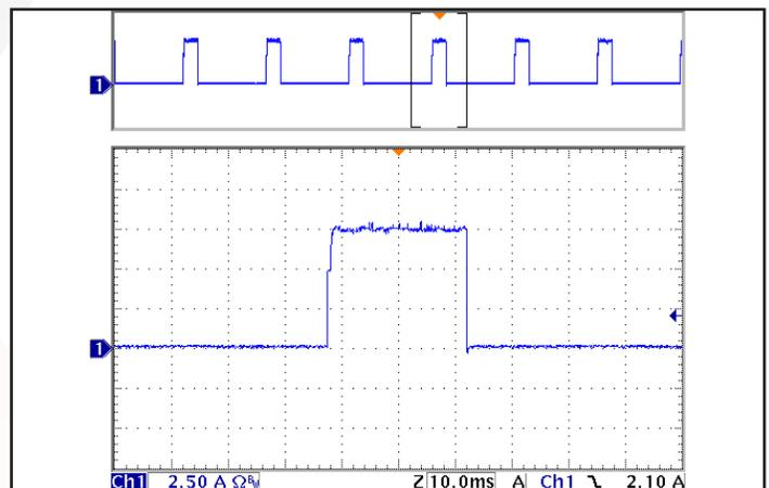
Figure 18: Load current (2.5A/div) as a function of time (10ms/div and 100ms/div) when the converter attempts to turn on into a  $1 \text{ m}\Omega$  short circuit.
