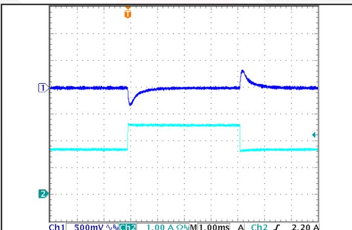
Figure 11: Output voltage response to step-change in load current (50-75-50% of  $I_{out(max)}$ ;  $di/dt = 0.1 A/\mu s$ ). Load cap: 1 µF ceramic and 100 µF electrolytic capacitors. Ch 1:  $V_{out}$  (500mV/div), Ch 2:  $I_{out}$  (1A/div). Timescale: 1.00ms/div.
