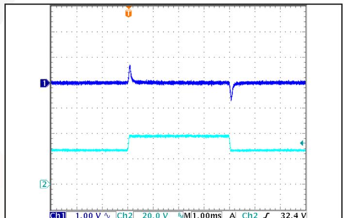
Figure 12: Output voltage response to step-change in input voltage (250V/ms). Load cap: 1µF ceramic and 15µF tantalum capacitance. Ch 1:  $V_{out}$  (1V/div), Ch 4:  $V_{in}$  (20V/div). Timescale: 1.00ms/div.
