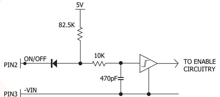
Figure A: Various circuits for driving the ON/OFF pin.
