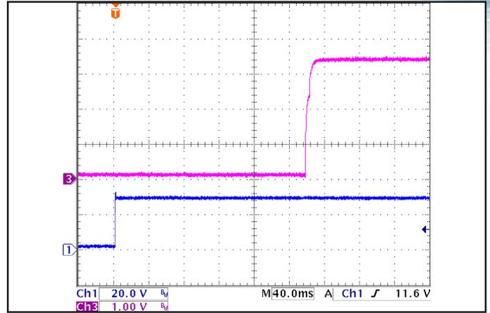
Figure 8: Turn-on transient at full resistive load and zero output capacitance initiated by Vin. ON/OFF Pin previously low. Ch 1: Vin (20V/div). Ch 3: Vout (1V/div).
