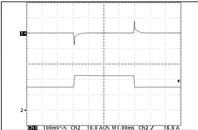
Figure 11: Output voltage response to step-change in load current (50%-75%-50% of  $I_{out(max)}$ );  $dI/dt = 0.1 A/\mu s$ . Load cap: 1 µF ceramic and 15 µF tantalum capacitors. Ch 1:  $V_{out}$  (100mV/div), Ch 2:  $I_{out}$  (10A/div).
