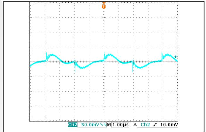
Figure 10: Output voltage ripple,  $V_{out}$ , at nominal input voltage and rated load current (50 mV/div). Load capacitance: 1µF ceramic capacitor and 15µF tantalum capacitor. Bandwidth: 10 MHz. See Figure 17.
