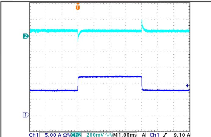
Figure 11: Output voltage response to step-change in load current (50-75-50% of  $I_{out(max)}$ ;  $di/dt = 0.1 A/\mu s$ ). Load cap: 1 µF ceramic and 100 µF electrolytic capacitors. Ch 1:  $I_{out}$  (5A/div), Ch 2:  $V_{out}$  (200mV/div). Timescale: 1.00ms/div.
