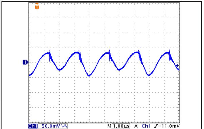
Figure 10: Output voltage ripple,  $V_{out}$ , at nominal input voltage and rated load current (50 mV/div). Load capacitance: 1µF ceramic capacitor and 15µF tantalum capacitor. Bandwidth: 20 MHz. Timescale: 1.00µsec/div. See Figure 17.
