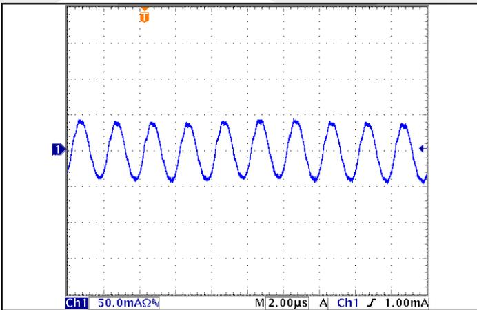
Figure 9: Input terminal current ripple,  $i_c$ , at full rated output current and nominal input voltage with SynQor MCOTS filter module (50 mA/div). Bandwidth: 20 MHz. Timescale: 2.00µs/div. See Figure 17.
