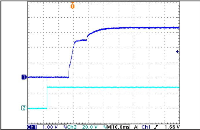
Figure 7: Turn-on transient at full load initiated by Nominal  $V_{in}$ . ON/OFF Pin previously low. Ch 1:  $V_{out}$  (1V/div). Ch 2:  $V_{in}$  (20V/div). Timebase: 10.0ms/div.
