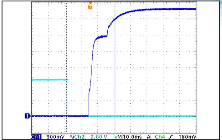
Figure 8: Typical startup waveform. Input voltage pre-applied, Ch 1:  $V_{out}$  (1V/div). Ch 2: ON/OFF Pin (5V/div). Timebase: 10.0ms/div.
