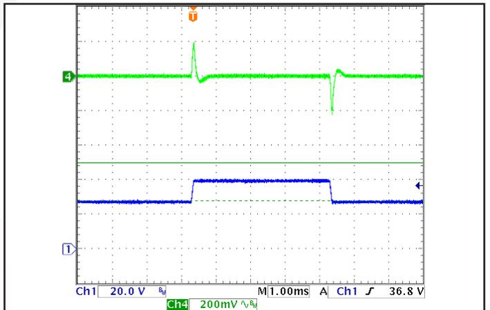
Figure 12: Output voltage response to step-change in input voltage (250V/ms). Load cap: 1µF ceramic and 15µF tantalum capacitance. Ch 1:  $V_{in}$  (20V/div), Ch 4:  $V_{out}$  (200mV/div). Timescale: 1.00ms/div.
