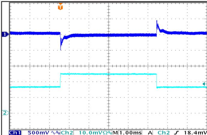
Figure 11: Output Voltage Response to Step-Change in Load Current (50%-75%-50% of  $I_{out(max)}$ );  $di/dt = 5 A/\mu s$ . Load cap: 1 µF ceramic and 100 µF electrolytic capacitors. Ch 1:  $V_{out}$  (500mV/div), Ch 2:  $I_{out}$  (10A/div).
