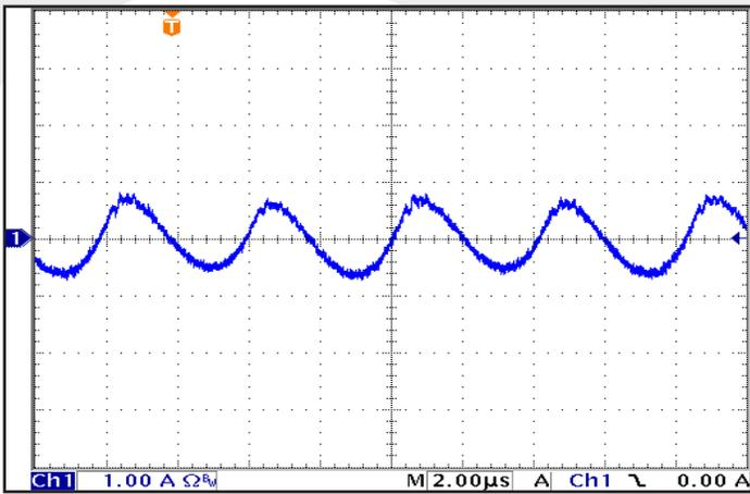
Figure 9: Input Terminal Current Ripple,  $i_{in}$ , at full rated output current and nominal input voltage with 3.3µH source impedance and 470µF electrolytic capacitor (1A/div). Bandwidth: 20MHz. See Figure 13.
