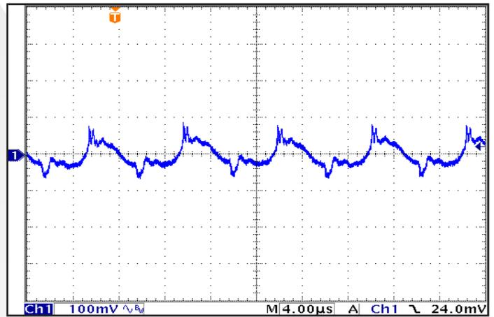
Figure 10: Output Voltage Ripple,  $V_{out}$ , at nominal input voltage and rated load current (100 mV/div). Load capacitance: 1µF ceramic capacitor and 100µF electrolytic capacitor. Bandwidth: 20 MHz. See Figure 13.
