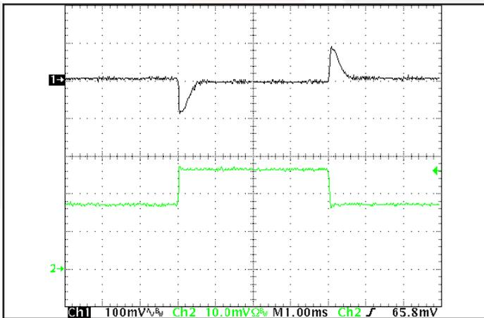
**Figure 11:** Output voltage response to step-change in load current (50%-75%-50% of  $I_{out(max)}$ ;  $dI/dt = 0.1 A/\mu s$ ). Load cap: 1 µF ceramic and 15 µF tantalum capacitors. Ch 1: Vout (100mV/div), Ch 2: Iout (5A/div).
