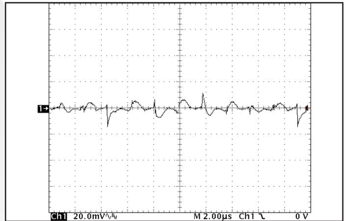
**Figure 10:** Output voltage ripple,  $V_{out}$ , at nominal input voltage and rated load current (20 mV/div). Load capacitance: 1µF ceramic capacitor and 10µF tantalum capacitor. Bandwidth: 10 MHz. See Figure 17.
