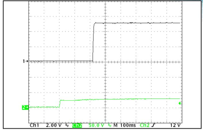
**Figure 8:** Turn-on transient at full resistive load and zero output capacitance initiated by Vin. ON/OFF Pin previously low. Ch 1: Vout (2V/div). Ch 3: Vin (50V/div).
