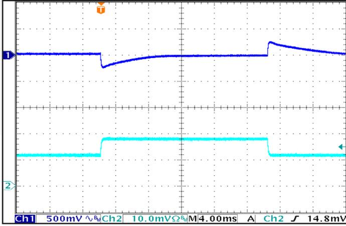
Figure 11: Output Voltage Response to Step-Change in Load Current (50%-75%-50% of  $I_{out(max)}$ ;  $di/dt = 0.1 A/\mu s$ ). Load cap: 1 µF ceramic and 100 µF electrolytic capacitors. Ch 1:  $V_{out}$  (500mV/div), Ch 2:  $I_{out}$  (20A/div).
