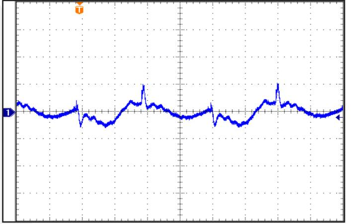
Figure 10: Output Voltage Ripple,  $V_{out}$ , at nominal input voltage and rated load current (50 mV/div). Load capacitance: 1µF ceramic capacitor and 100µF electrolytic capacitor. Bandwidth: 20 MHz. See Figure 13.
