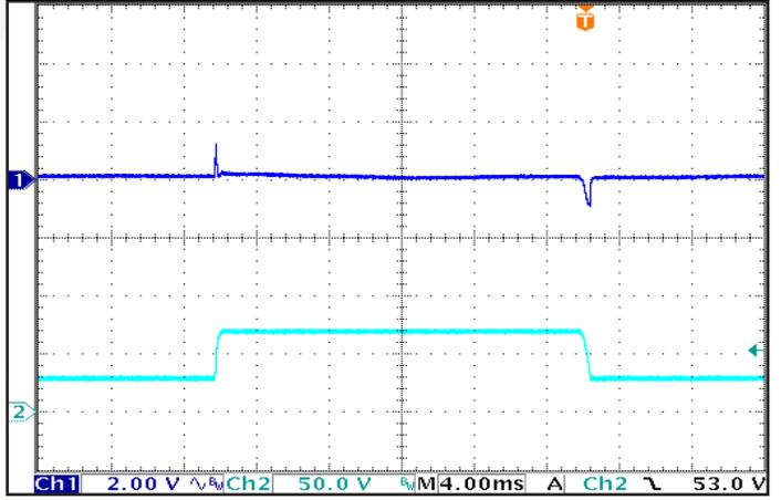
Figure 12: Output Voltage Response to Step-Change in Input Voltage (250V/ms). Load cap: 330 µF electrolytic output capacitance. Ch 1:  $V_{out}$  (2V/div), Ch 2:  $V_{in}$  (50V/div).
