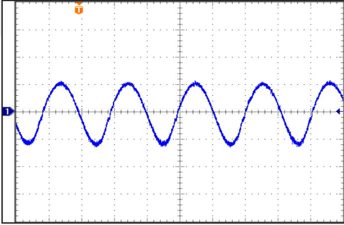
Figure 9: Input Terminal Current Ripple,  $i_{in}$ , at full rated output current and nominal input voltage with SynQor MCOTS filter module (2 A/div). Bandwidth: 20MHz. See Figure 13.
