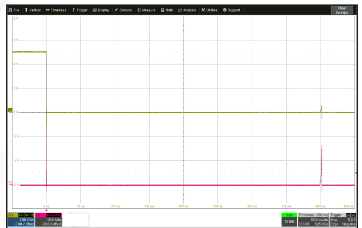
Figure 18: A short circuit across the output terminals. Ch 1: V_{out} (2 V/div). Ch 2: I_{out} (10 A/div). Timecale: 50.0 ms/div.
