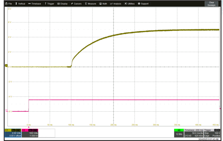
Figure 8: Turn-on transient at full load and zero output capacitance initiated by V_{in} . On/Off Pin previously low. Ch 1: V_{out} (2 V/div). Ch 2: V_{in} (500 V/div). Timescale: 50.0 ms/div.
