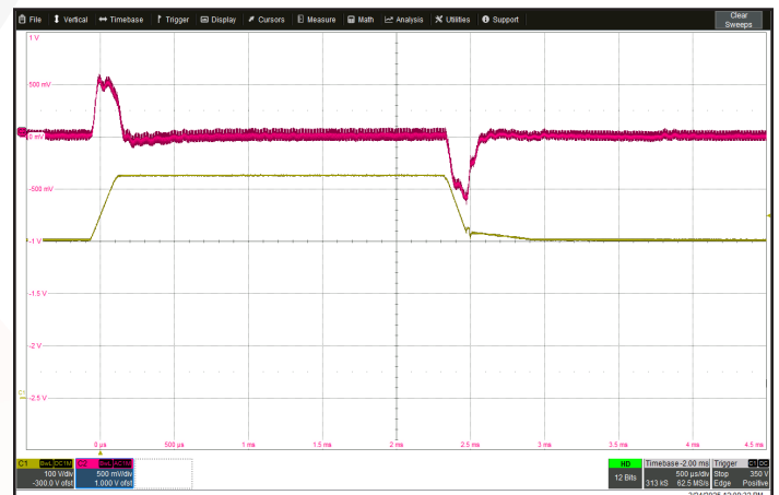
Figure 12: Output voltage response to step-change in input voltage (300 V - 425 V) in 125 \mu s. Ch 1: V_{in} (100 V/div). Ch 2: V_{out} (500 mV/div). Timescale: 500 \mu s/div.
