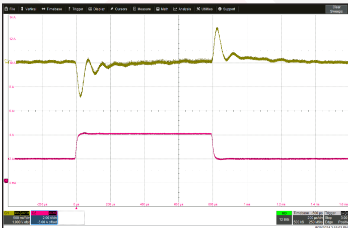
Figure 11: Output voltage response to step-change in load current 50%-100%-50% of I_{out} (max). No external load capacitance. Ch 1: V_{out} (500 mV/div). Ch 2: I_{out} (2 A/div). Timescale: 200 μs/div.
