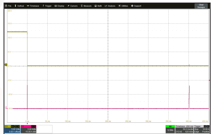
Figure 18: A short circuit across the output terminals. Ch 1: V_{out} (5 V/div). Ch 2: I_{out} (5 A/div). Timecale: 50.0 ms/div.
