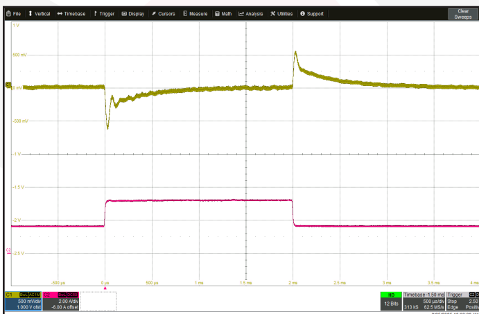
Figure 11: Output voltage response to step-change in load current 50%-100%-50% of I_{out} (max). No external load capacitance. Ch 1: V_{out} (500 mV/div). Ch 2: I_{out} (2 A/div). Timescale: 500 \mu s/div.
