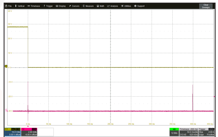
Figure 18: A short circuit across the output terminals. Ch 1: V_{out} (10 V/div). Ch 2: I_{out} (2 A/div). Timecale: 50.0 ms/div.
