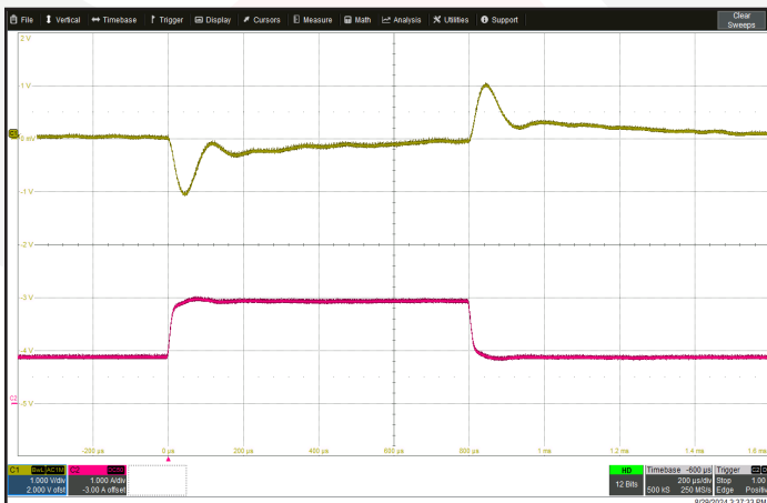
Figure 11: Output voltage response to step-change in load current 50%-100%-50% of Iout (max). No external load capacitance. Ch 1: Vout (1 V/div). Ch 2: Iout (1 A/div) Timescale: 200 μs/div.
