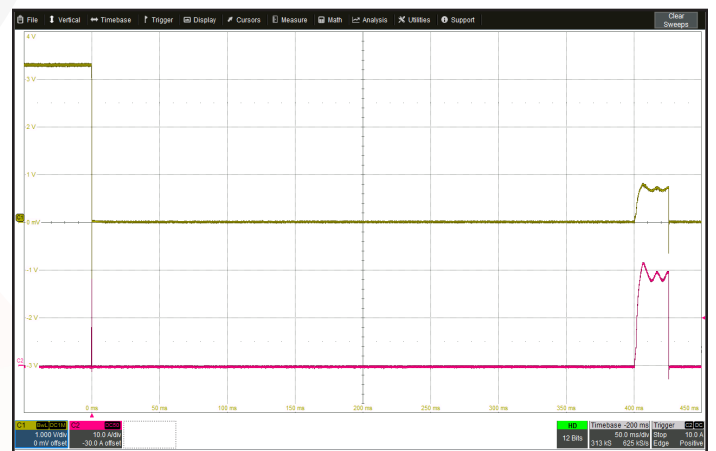
Figure 18: A short circuit across the output terminals. Ch 1: V_{out} (1 V/div). Ch 2: I_{out} (10 A/div). Timecale: 50.0 ms/div.
