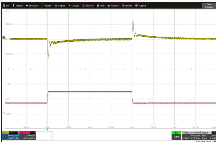
Figure 11: Output voltage response to step-change in load current 50%-100%-50% of Iout (max). No external load capacitance. Ch 1: Vout (500 mV/div). Ch 2: Iout (10 A/div). Timescale: 500 μs/div.
