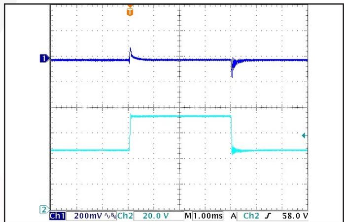
**Figure 12:** Output voltage response to step-change in input voltage (1000V/ms). Ch 1: Vout (200mV/div), Ch 2: Vin (20V/div).
