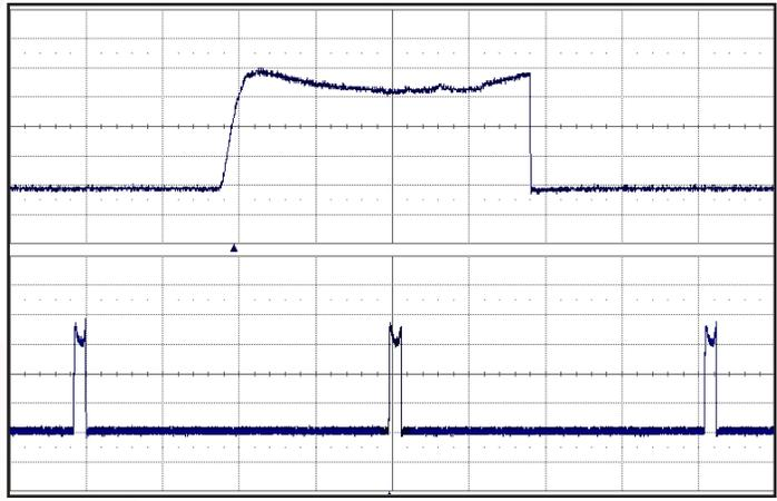
Figure 18: Load current (10A/div) as a function of time (1ms/div and 50ms/div) when the converter attempts to turn on into a 10 mΩ short circuit.
