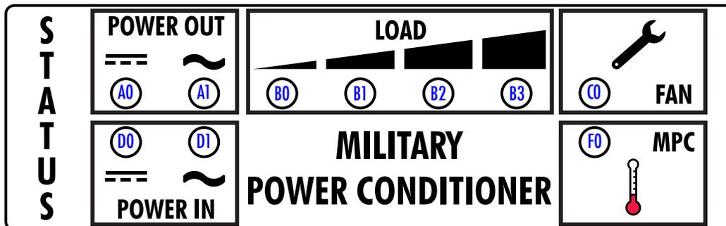
**LEDs on the Front Panel - “Constant Current” Model**
