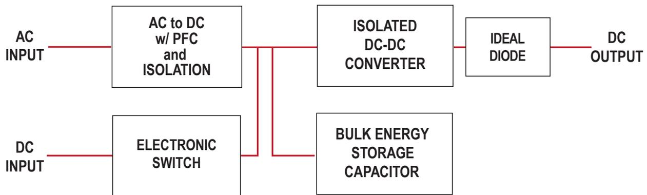
Power flows from the AC INPUT through an AC-DC converter that has Power Factor Correction (PFC) and high-frequency safety isolation. Power flows from the DC INPUT through an electronic switch that is closed when the AC INPUT power is absent and the DC INPUT voltage is within its specified range.
