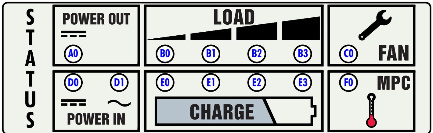
LEDs E0 – E3 provide a visual representation of the output voltage level. When the output voltage is close to the nominal ( $V_{set}$ ), all four LEDs will be illuminated green. When the output voltage is below 21 V, LED E0 will be amber and E1-E3 will be off.
