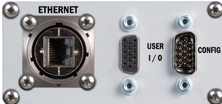
The User I/O female DB15 connector on the left is for a connection to a host/system computer so that it can control the MPC and receive information regarding the status of the MPC.
