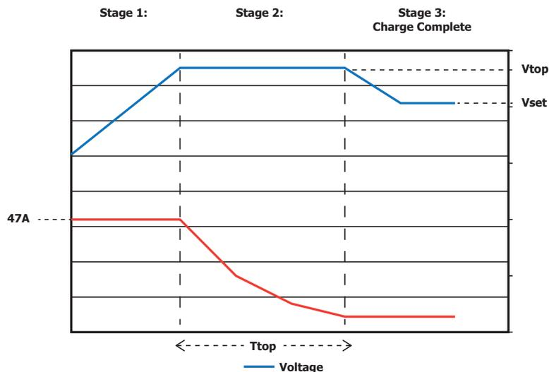
During Stage I, the battery charges with a Constant Current (CC). The MPC-1250 can supply 47 A in constant current mode. If no loads are active, the battery will charge with 47 A. If loads are active, the battery charge current will be reduced by the load current.
