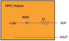
The purpose of the AUX power supply is to provide a low level of power to control circuitry at the output of the MPFCQor, such as the circuits shown earlier in this section.
