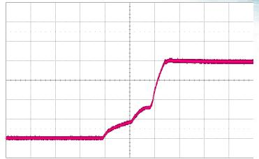
*Figure 8*: Output voltage startup waveform with 200uF hold-up capacitor, no load (115VAC, 60Hz) Vout (100V/div), Timebase: (500ms/div)
