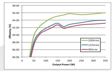
**Figure 1:** Efficiency at nominal output voltage vs. load power for 90Vrms, 115Vrms and 230Vrms (60Hz) input voltage at Tb = 25 °C.
