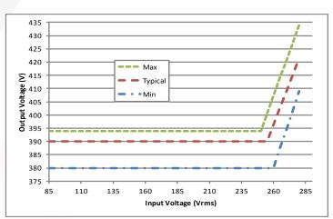
Figure 6: DC output voltage range vs. input voltage
