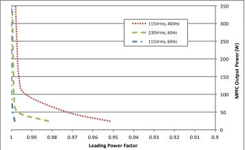
Figure 5: Output power vs. leading power factor, MPFC module only
