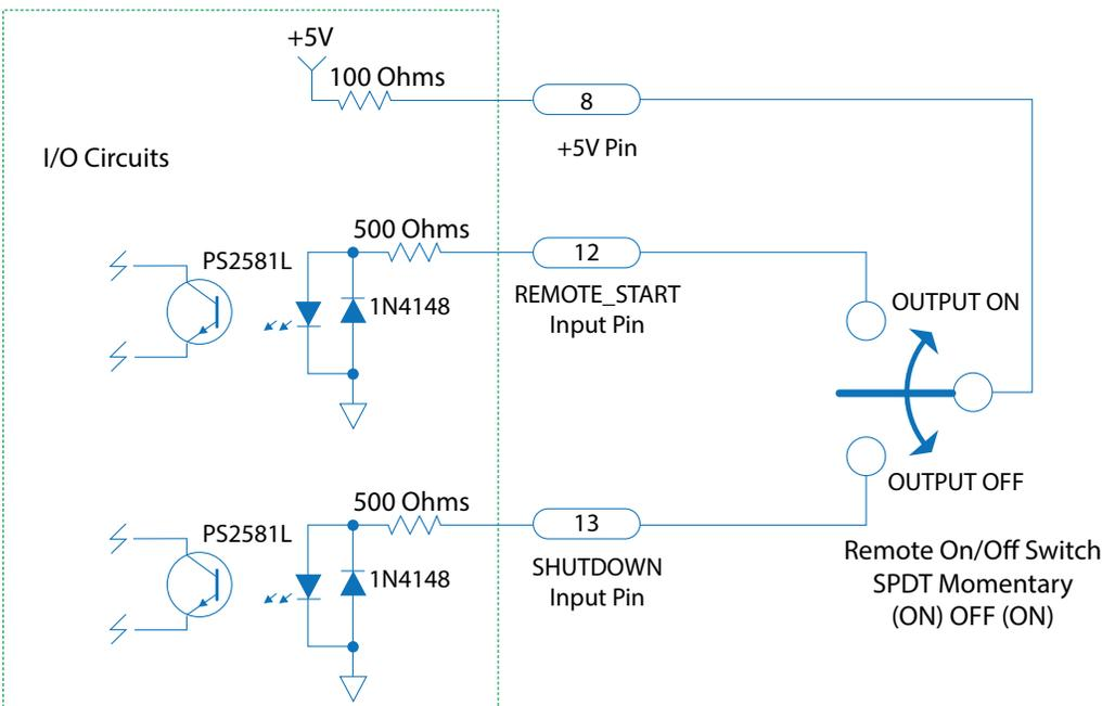
Note: A 2PDT or 3PDT switch may be substituted for single control of 2 or 3 MPPS machines, respectively.
