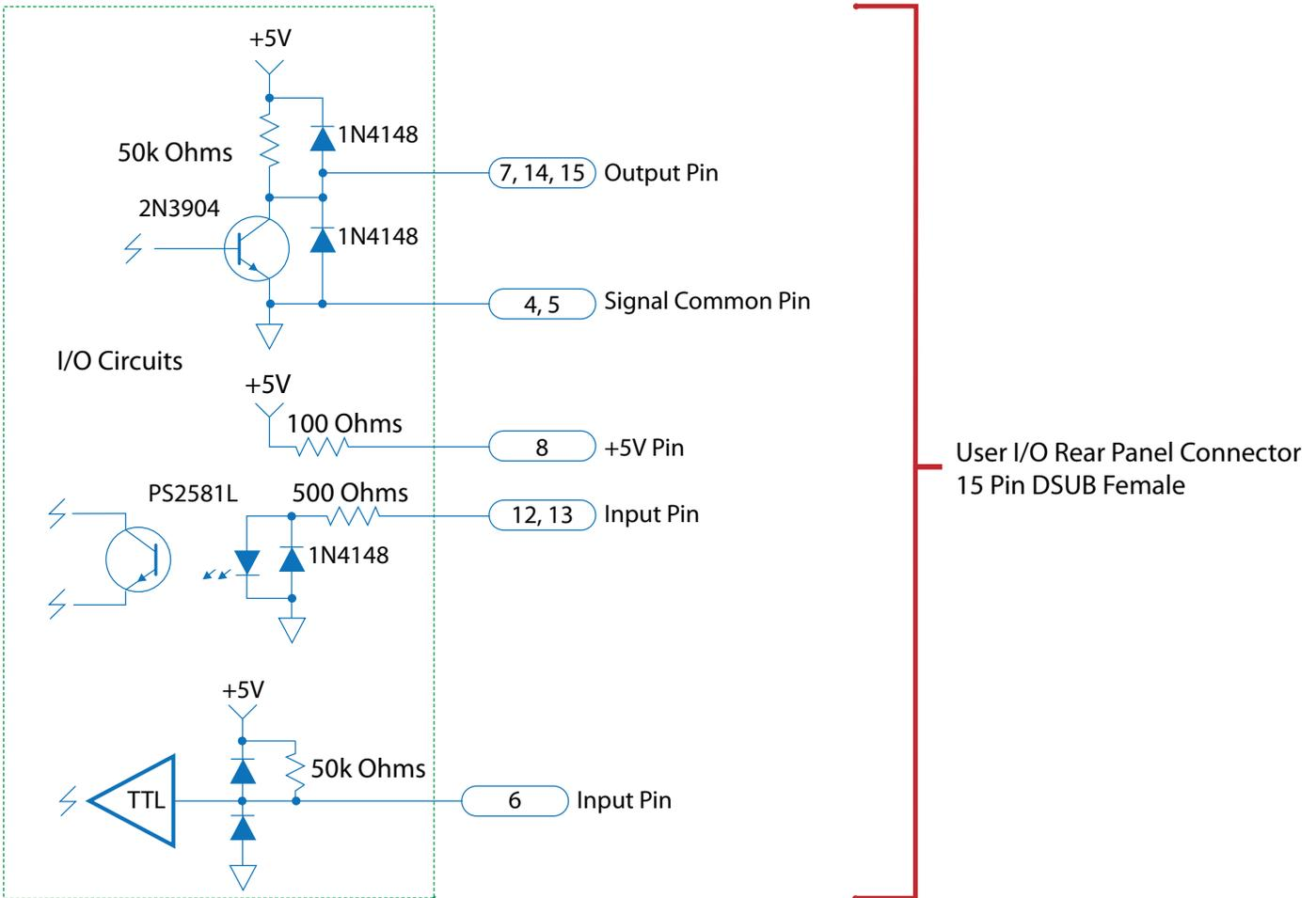
**Remote On/Off Switch Connections**
