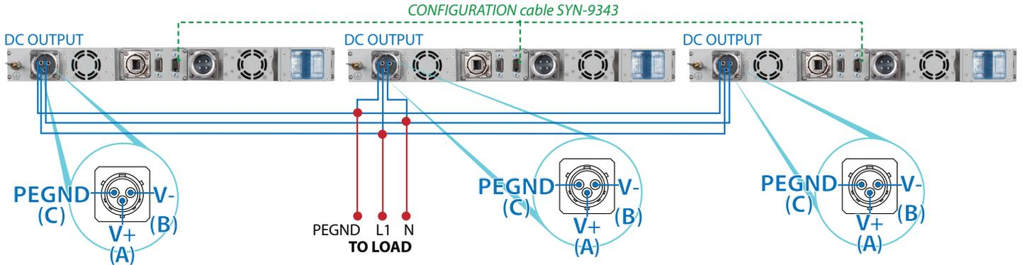
If the user is providing its own DC OUTPUT cable, the size of the blue and red cable sections shown above, should follow the guidelines shown in the table below depending on DC OUTPUT voltage of the MPPS units.
