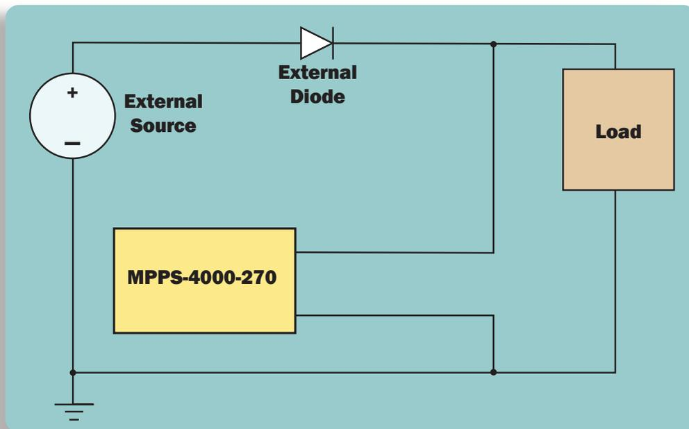
*MPPS diode ORing with 3<sup>rd</sup> party auxiliary supply*
