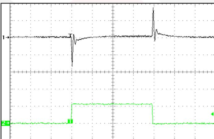
**Figure 11:** Output voltage response to step-change in load current 0%-50%-0% of Iout (max). Load cap: 1uF ceramic cap and 10uF, 100mOhm ESR tantalum cap. Ch 1: Vout (200mV/div). Ch 2: Iout (1A/div).
