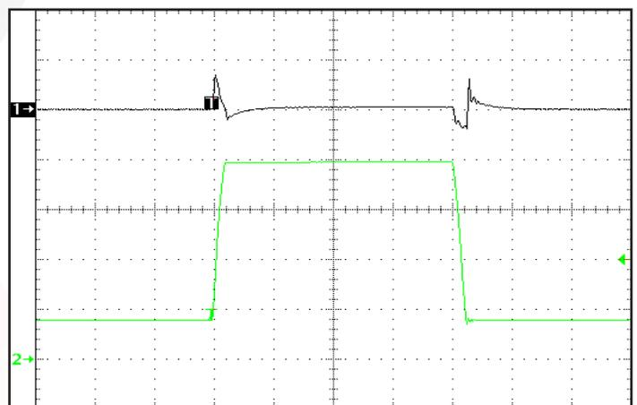
**Figure 12:** Output voltage response to step-change in input voltage (16V - 80V - 16V) in 150uS. Ch 1: Vout (100mV/div). Ch 2: Vin (20V/div).
