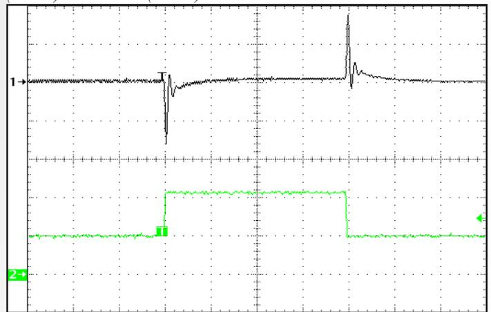
**Figure 10:** Output voltage response to step-change in load current 50%-100%-50% of Iout (max). Load cap: 1uF ceramic cap and 10uF, 100mOhm ESR tantalum cap. Ch 1: Vout (200mV/div). Ch 2: Iout (1A/div).
