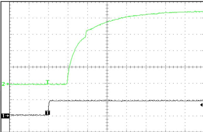
**Figure 7:** Turn-on transient at full resistive load and zero output capacitance initiated by ENA1. Input voltage pre-applied. Ch 1: ENA1 (5V/div). Ch 2: Vout (2V/div).
