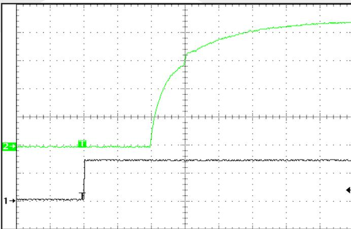
**Figure 9:** Turn-on transient at full resistive load and zero output capacitance initiated by Vin. ENA1 previously high. Ch 1: Vin (20V/div). Ch 2: Vout (2V/div).
