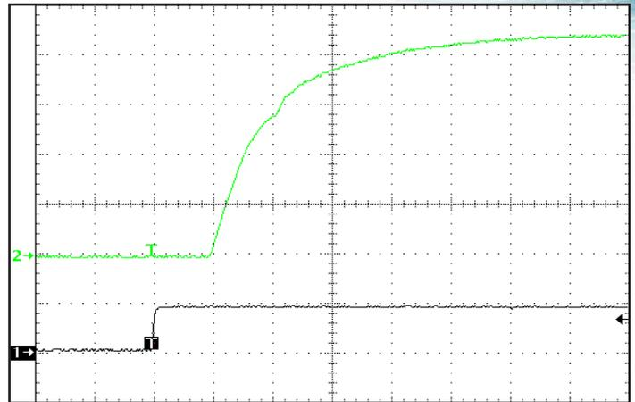
**Figure 8:** Turn-on transient at full resistive load and 600uF output capacitance initiated by ENA1. Input voltage pre-applied. Ch 1: ENA1 (5V/div). Ch 2: Vout (2V/div).
