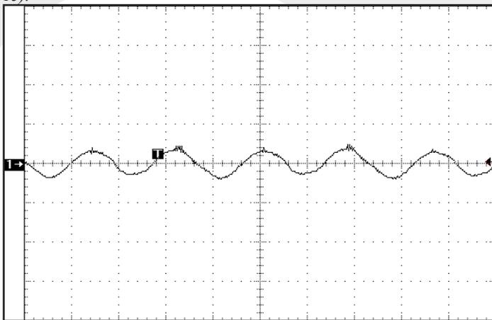
**Figure 15:** Output voltage ripple,  $V_{out}$ , at nominal input voltage and rated load current (20mV/div). Load capacitance: 1µF ceramic capacitor and 10µF tantalum capacitor. Bandwidth: 10MHz. See Figure 13.
