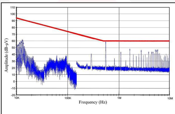
**Figure 22:** High frequency conducted emissions of standalone MQHL-28-05S, 5V<sub>out</sub> module at 50W output, as measured with Method CE102. Limit line shown is the 'Basic Curve' for all applications with a 28V source.
