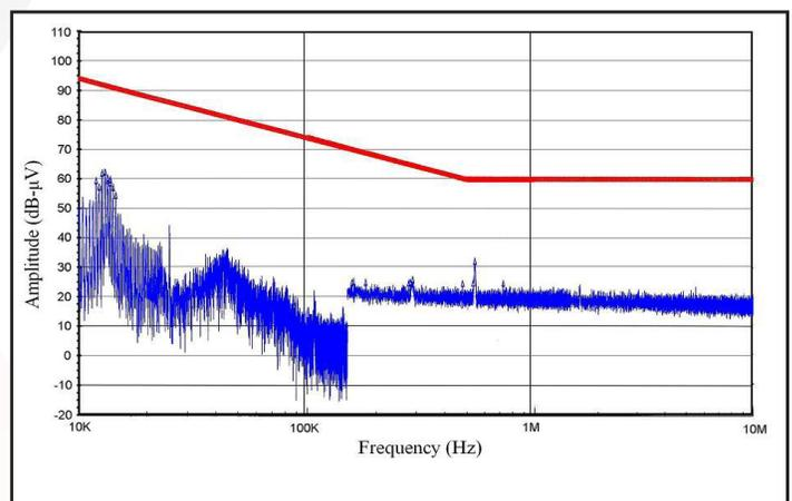
**Figure 23:** High frequency conducted emissions of MQHL-28-05S, 5V<sub>out</sub> module at 50W output with MQHE-28-P filter, as measured with Method CE102. Limit line shown is the 'Basic Curve' for all applications with a 28V source.
