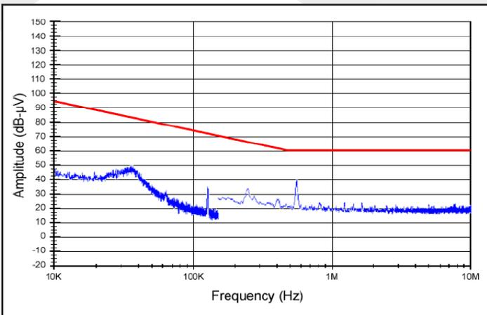
Figure 33: High frequency conducted emissions of MQFL-270-05S, 5V<sub>out</sub> module at 120W output with MQME-270-P filter, as measured with Method CE102. Limit line shown is the 'Basic Curve' for all applications with a 270V source.
