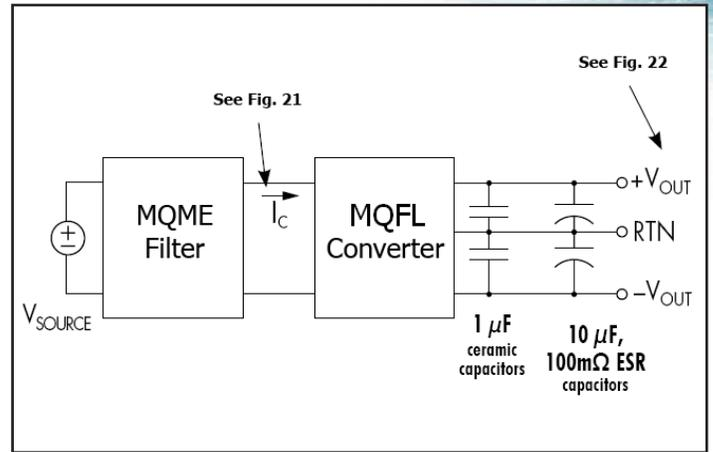
Figure 20: Test set-up diagram showing measurement points for Input Terminal Ripple Current (Fig 21) and Output Voltage Ripple (Fig 22).
