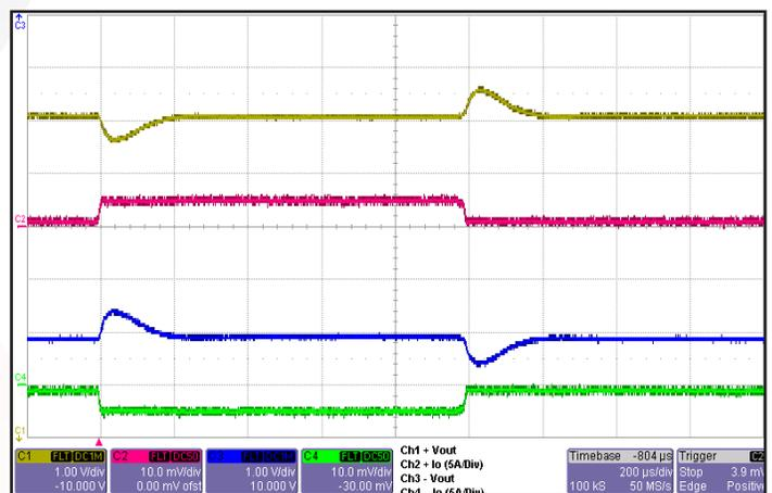
Figure 18: Output voltage response to step-change in total load current (10%-50%-10%) of total Iout (max) split 50%/50%. Load cap: 1µF ceramic cap and 10µF, 100 mW ESR tantalum cap. Ch 1: +Vout (1 V/div); Ch 2: +Iout (5A/div); Ch 3: -Vout (1 V/div); Ch 4: -Iout (5A/div).
