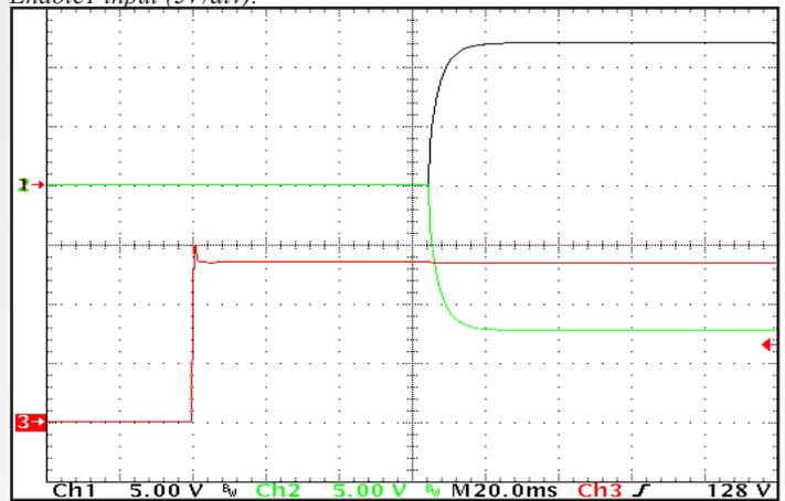
Figure 16: Turn-on transient at full load, after application of input voltage (ENA 1 and ENA 2 logic high) (5 ms/div). Ch 1: +Vout (5V/div); Ch 2: -Vout (5V/div); Ch 3: Vin (100V/div).
