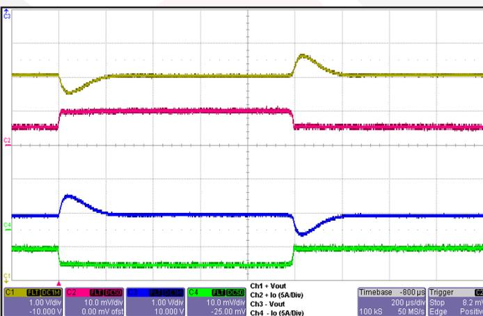
Figure 17: Output voltage response to step-change in total load current (50%-100%-50%) of total Iout (max) split 50%/50%. Load cap: 1µF ceramic cap and 10µF, 100mW ESR tantalum cap. Ch 1: +Vout (1 V/div); Ch 2: +Iout (5A/div); Ch 3: -Vout (1 V/div); Ch 4: -Iout (5A/div).
