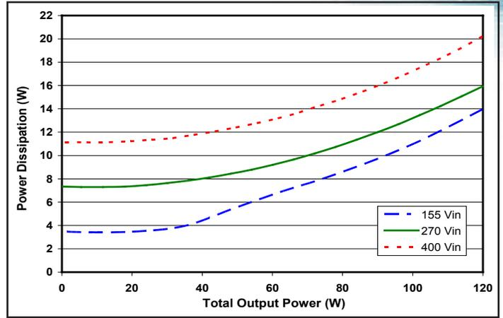
Figure 1: Efficiency vs. output power, from zero load to full load with equal load on the +12V output and 50% load on the -12V output at minimum, nominal, and maximum input voltage at 25°C.
