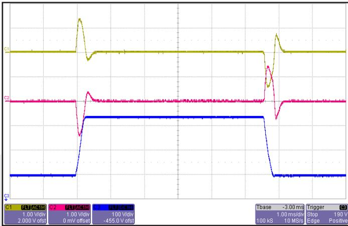
Figure 19: Output voltage response to step-change in input voltage (155V - 400V - 155V). Load cap: 10µF, 100 mW ESR tantalum cap and 1µF ceramic cap. Ch 1: +Vout (1V/div); Ch 2: -Vout (1V/div); Ch 3: Vin (100V/div).
