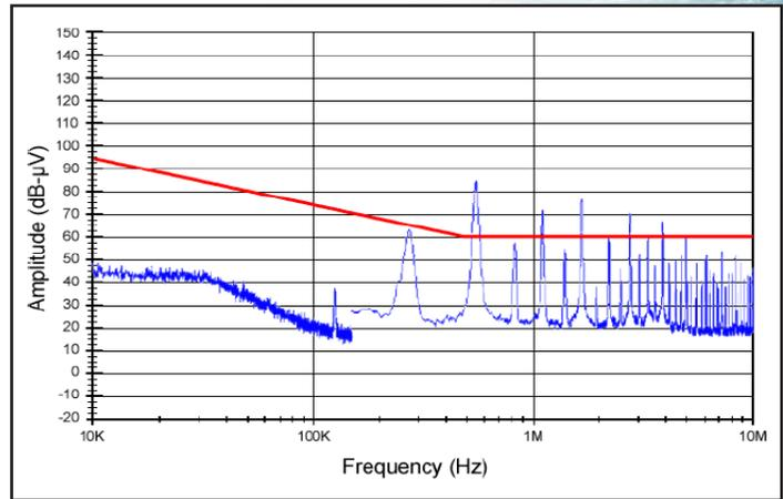
Figure 32: High frequency conducted emissions of standalone MQFL-270-05S, 5V<sub>out</sub> module at 120W output, as measured with Method CE102. Limit line shown is the 'Basic Curve' for all applications with a 270V source.
