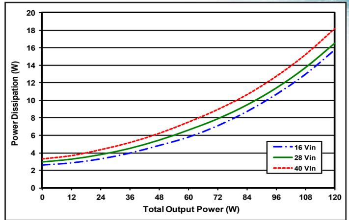
Figure 2: Power dissipation vs. output power, from zero to full load with equal load on the +5V and -5V outputs at minimum, nominal, and maximum input voltage at 25°C.
