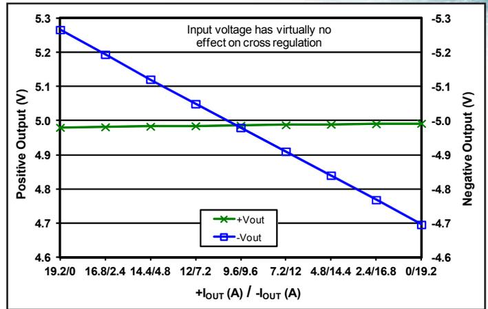
Figure 8: Load regulation vs. load current with power fixed at 80% load (96 W) and load currents split as shown between the +5V and -5V outputs, at nominal input voltage and  $T_{case} = 25^{\circ}C$ .
