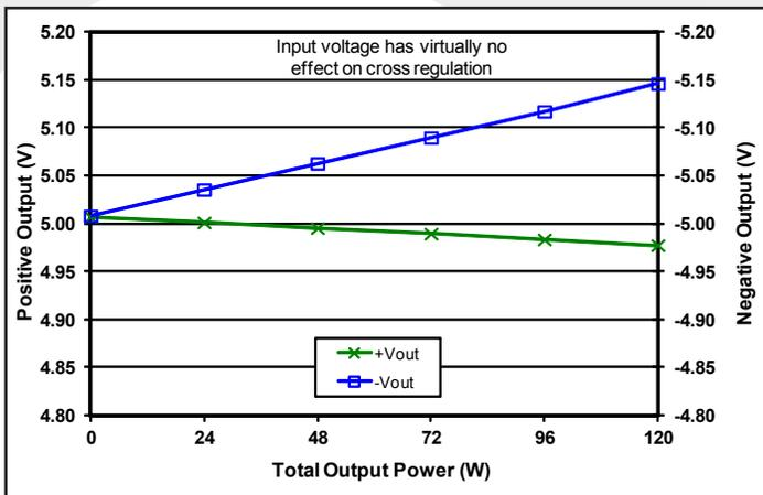
Figure 9: Load regulation vs. total output power from zero to full load where  $+I_{out}$  equals three times  $-I_{out}$  at nominal input voltage and  $T_{case} = 25^{\circ}C$ .
