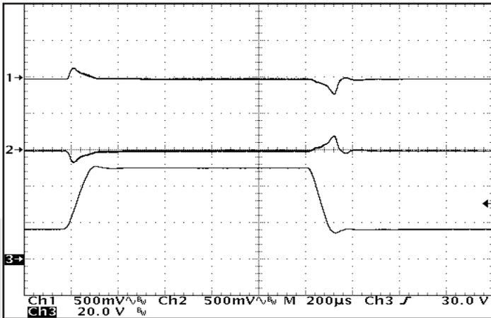
Figure 19: Output voltage response to step-change in input voltage (16V-50V-16V). Load camp: 10µF, 100 mΩ ESR tantalum cap and 1µF ceramic cap. Ch 1: +Vout (500mV/div); Ch 2: -Vout (500mV/div); Ch 3: Vin (20V/div).
