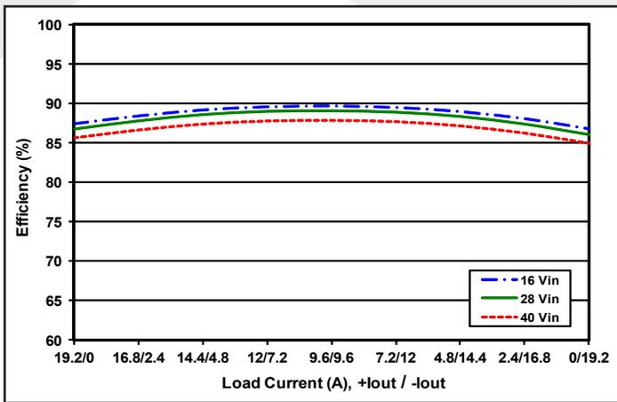
Figure 3: Efficiency vs. output current, with total output current fixed at 80% load (96 W) and loads split as shown between the +5V and -5V outputs at minimum, nominal, and maximum input voltage at 25°C.
