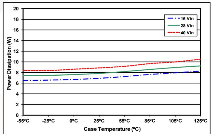
Figure 6: Power dissipation at 60% load (7.2 A load on +5V and 7.2 A load on -5V) versus case temperature for Vin = 16V, 28V, and 40V.
