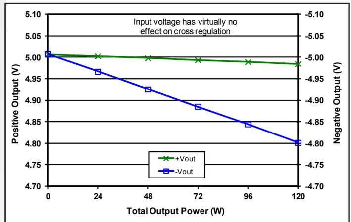
Figure 10: Load regulation vs. total output power from zero to full load where  $-I_{out}$  equals three times  $+I_{out}$  at nominal input voltage and  $T_{case} = 25^{\circ}C$ .
