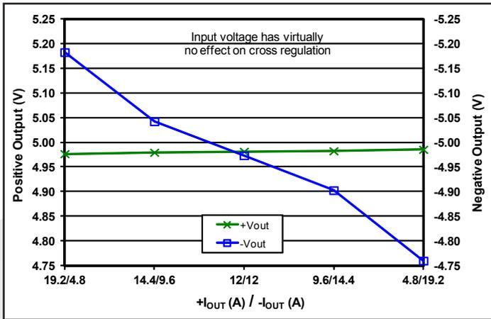
Figure 7: Load regulation vs. load current with power fixed at full load (120 W) and load currents split as shown between the +5V and -5V outputs, at nominal input voltage and  $T_{case} = 25^{\circ}C$ .
