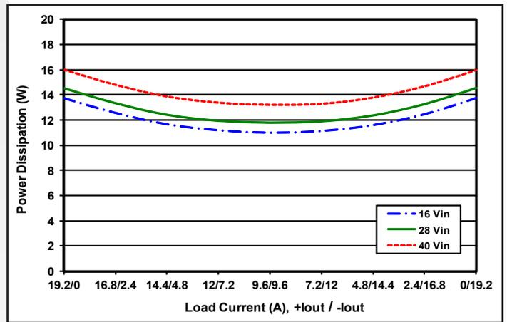
Figure 4: Power dissipation vs. output current, with total output current fixed at 80% load (96 W) and loads split as shown between the +5V and -5V outputs at minimum, nominal, and max input voltage at 25°C.
