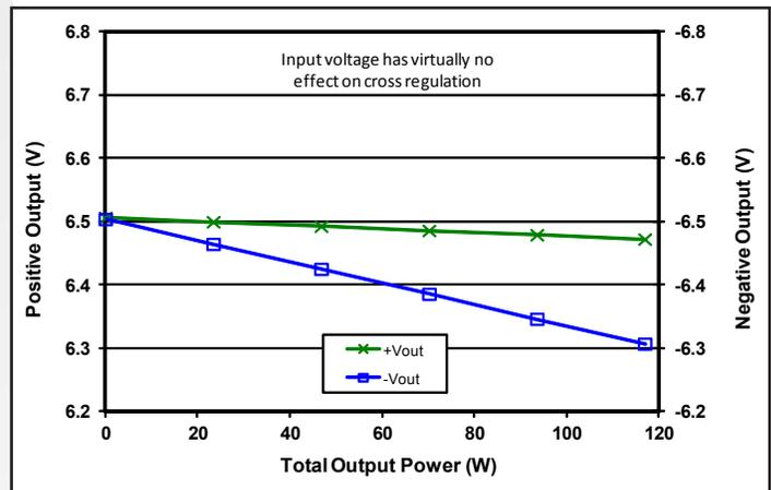
Figure 10: Load regulation vs. total output power from zero to to full load where -I<sub>out</sub> equals three times +I<sub>out</sub> at nominal input voltage and T<sub>case</sub> = 25 °C.
