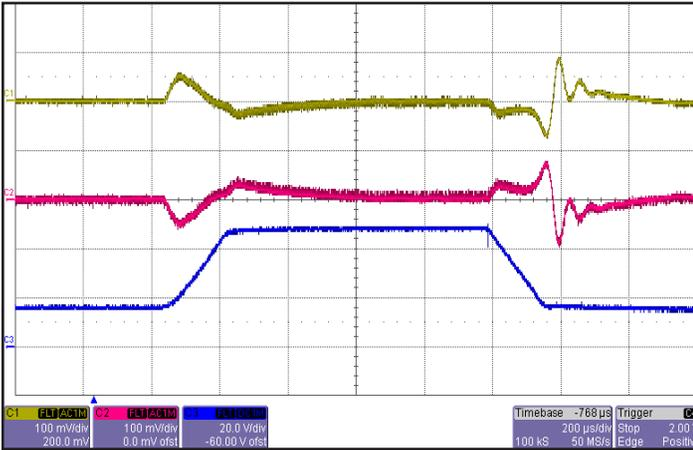
Figure 19: Output voltage response to step-change in input voltage (16 V - 50 V - 16 V). Load cap: 10  $\mu$ F, 100 m $\Omega$  ESR tantalum cap and 1  $\mu$ F ceramic cap. Ch 1: +Vout (100 mV/div); Ch 2: -Vout (100 mV/div); Ch 3: Vin (20 V/div).
