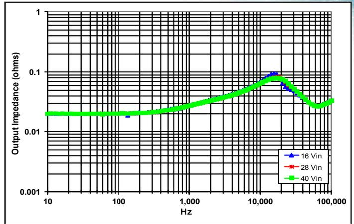
Figure 25: Magnitude of incremental output impedance of +6.5 V output (+Zout = +vout /+iout) for minimum, nominal, and maximum input voltage at full rated power.
