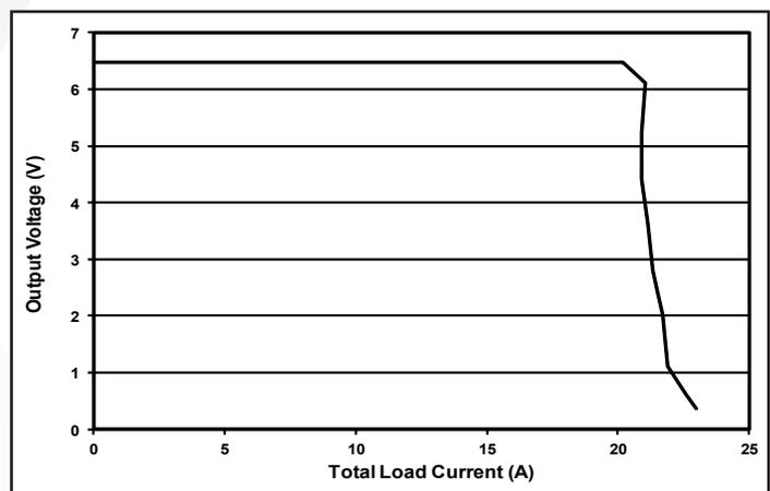
Figure 12: Positive output voltage vs. total load current, evenly split, showing typical current limit curves at V<sub>in</sub> = 28 V.
