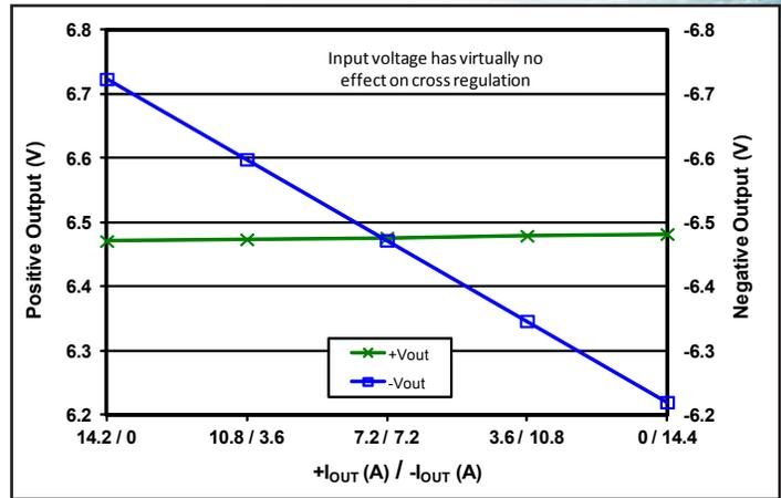
Figure 8: Load regulation vs. load current with power fixed at 80% load (93.6 W) and load currents split as shown between the +6.5 V and -6.5 V outputs, at nominal input voltage and T<sub>case</sub> = 25 °C.
