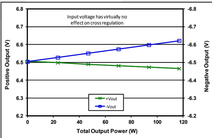
Figure 9: Load regulation vs. total output power from zero to to full load where +I<sub>out</sub> equals three times -I<sub>out</sub> at nominal input voltage and T<sub>case</sub> = 25 °C.
