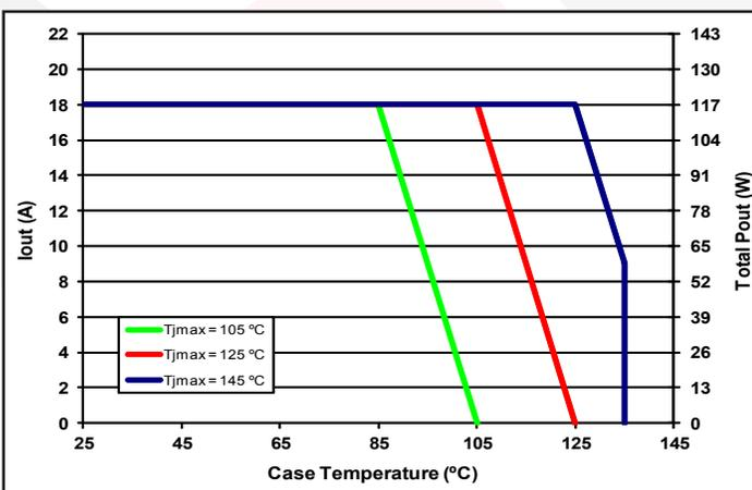
Figure 11: Total Output Current / Total Output Power derating curve as a function of T<sub>case</sub> and the maximum desired power MOSFET junction temperature at V<sub>in</sub> = 28 V (see Note 15).
