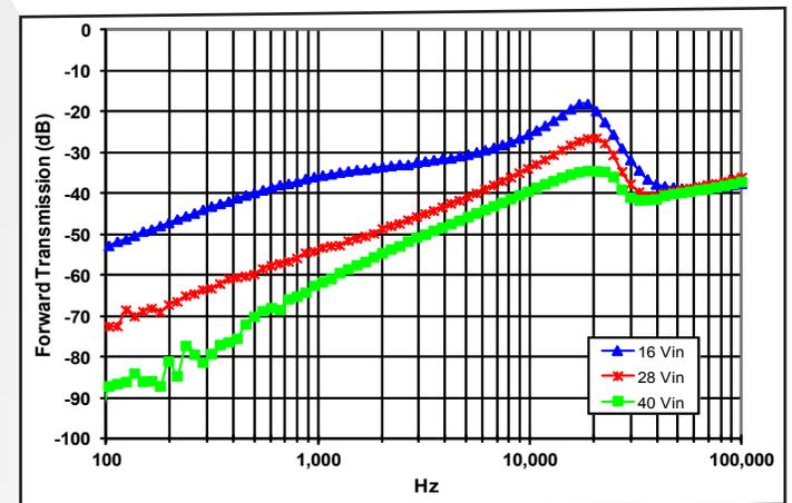
Figure 27: Magnitude of incremental forward transmission of +6.5 V output (+FT = +vout /vin) for minimum, nominal, and maximum input voltage at full rated power.
