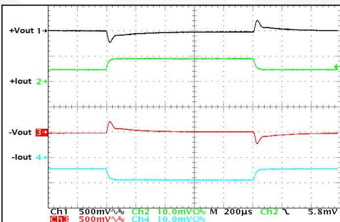
Figure 17: Output voltage response to step-change in total load current (50%-100%-50%) of total Iout (max) split 50%/50%. Load cap: 1 µF ceramic cap and 10 µF, 100 mΩ ESR tantalum cap. Ch 1: +Vout (500 mV/div); Ch 2: +Iout (10 A/div); Ch 3: -Vout (500 mV/div); Ch 4: -Iout (10 A/div).
