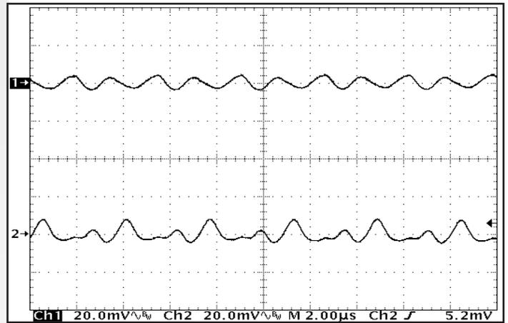
Figure 22: Output voltage ripple, +Vout (Ch 1) and -Vout (Ch 2), at nominal input voltage and full load current evenly split (20 mV/div). Load capacitance: 1  $\mu$ F ceramic cap and 10  $\mu$ F tantalum cap. Bandwidth: 10 MHz. See Figure 20.
