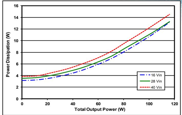
Figure 1: Efficiency vs. output power, from zero load to full load with equal load on the +6.5 V and -6.5 V outputs at minimum, nominal, and maximum input voltage at 25 °C.
