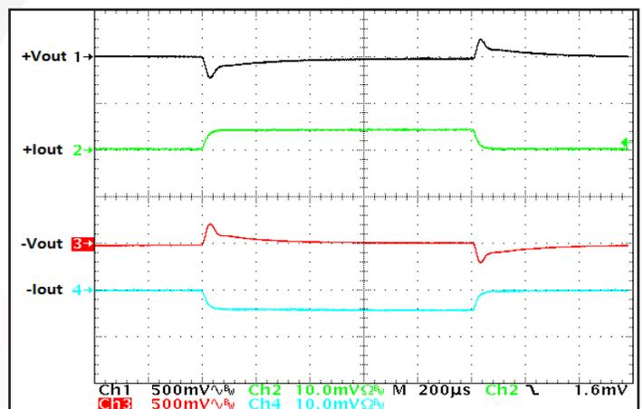
Figure 18: Output voltage response to step-change in total load current (0%-50%-0%) of total Iout (max) split 50%/50%. Load cap: 1 µF ceramic cap and 10 µF, 100 mΩ ESR tantalum cap. Ch 1: +Vout (500 mV/div); Ch 2: +Iout (10 A/div); Ch 3: -Vout (500 mV/div); Ch 4: -Iout (10 A/div).
