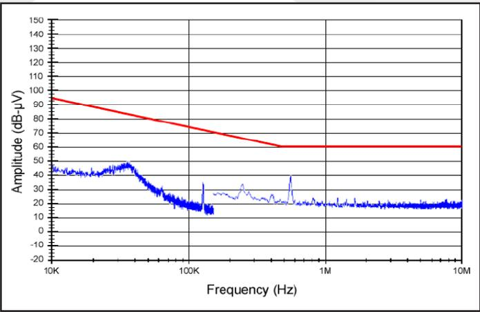
Figure 33: High frequency conducted emissions of MQFL-28-05S, 5 Vout module at 120 W output with MQFL-28-P filter, as measured with Method CE102. Limit line shown is the 'Basic Curve' for all applications with a 28 V source.
