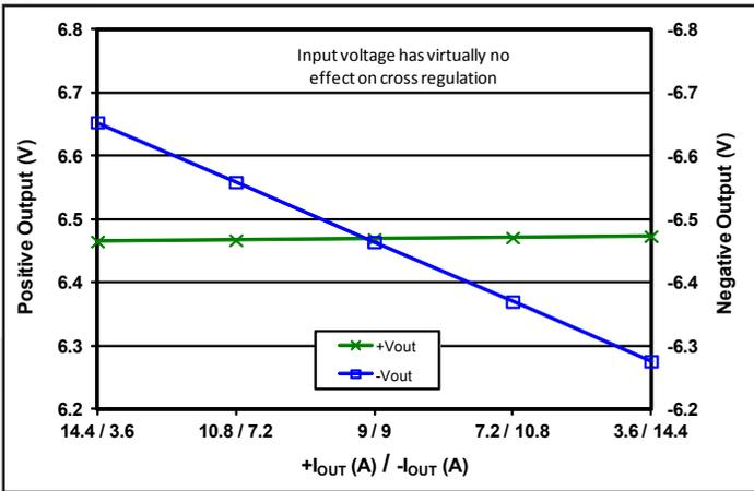
Figure 7: Load regulation vs. load current with power fixed at full load (117 W) and load currents split as shown between the +6.5 V and -6.5 V outputs, at nominal input voltage and T<sub>case</sub> = 25 °C.
