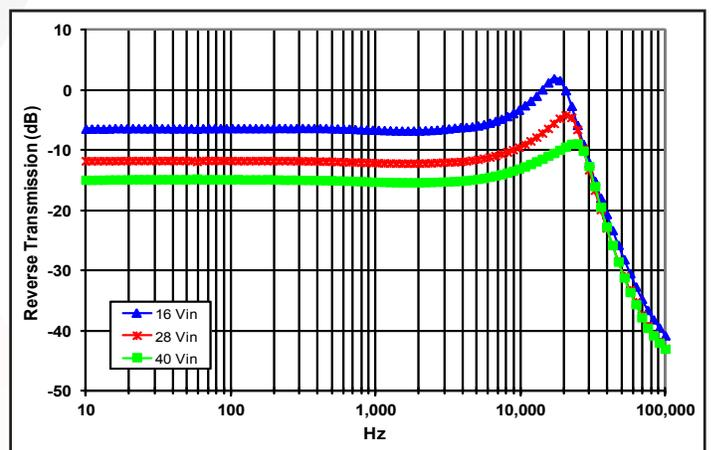
Figure 29: Magnitude of incremental reverse transmission from +6.5 V output (+RT = iin /+iout) for minimum, nominal, and maximum input voltage at full rated power.
