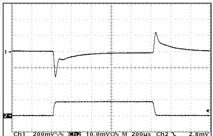
Figure 12: Output voltage response to step-change in load current (0%-50%-0%) of  $I_{out(max)}$ . Load cap: 1  $\mu$ F ceramic cap and 10  $\mu$ F, 100 mW ESR tantalum cap. CH1: Vout (200 mV/div). CH2: Iout (10 A/div).  $V_{in}=28$  V.
