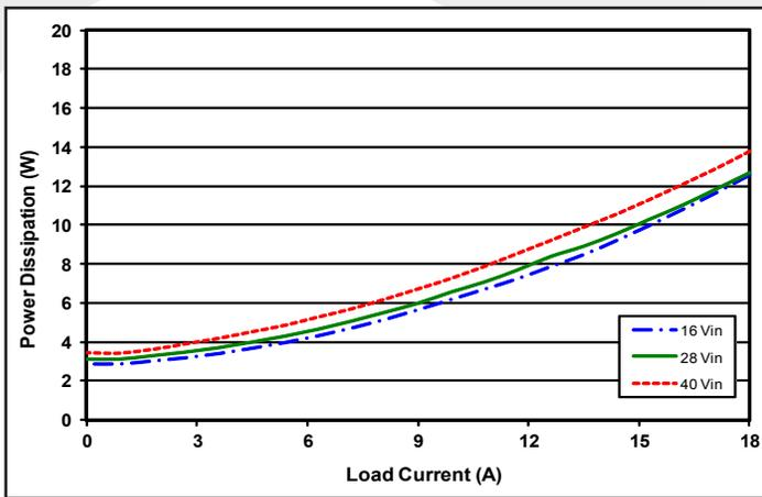
Figure 3: Power dissipation at nominal output voltage vs. load current for minimum, nominal, and maximum input voltage at  $T_{case}=25\text{ }^{\circ}\text{C}$ .
