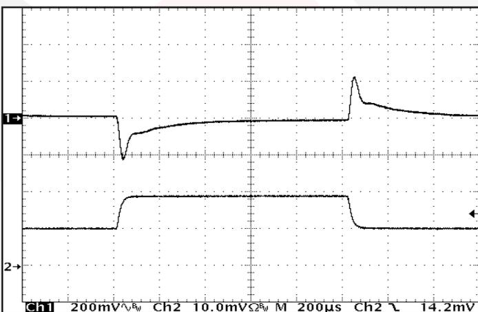
Figure 11: Output voltage response to step-change in load current 50%-100%-50% of  $I_{out(max)}$ . Load cap: 1  $\mu$ F ceramic cap and 10  $\mu$ F, 100 mohm tantalum cap. CH1: Vout (200 mV/div). CH2: Iout (10 A/div).  $V_{in}=28$  V.
