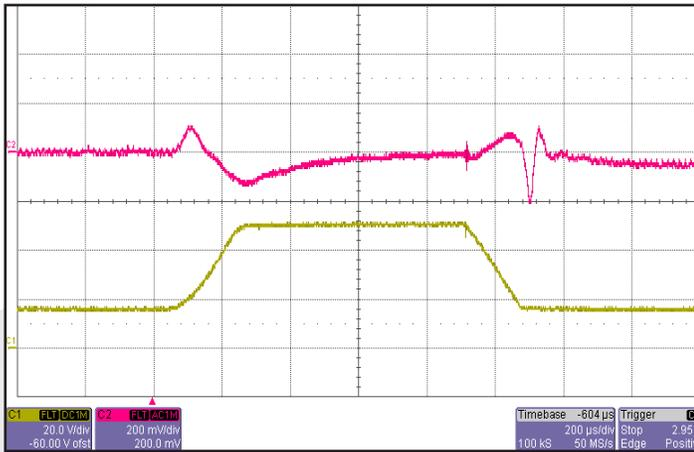
Figure 13: Output voltage response to step-change in input voltage (16 V-50 V-16 V). Load cap: 10  $\mu$ F m $\Omega$  ESR tantalum cap and 1  $\mu$ F ceramic cap. Ch 1:  $V_{in}$  (20 V/div). Ch 2:  $V_{out}$  (200 mV/div).
