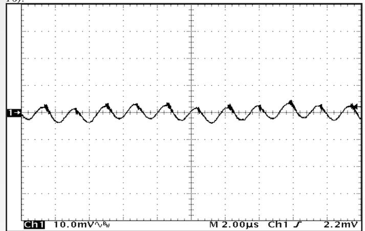
Figure 16: Output voltage ripple,  $V_{out}$  at nominal input voltage and rated load current (10 mV/div). Load capacitance: 1  $\mu$ F ceramic capacitor and 10  $\mu$ F tantalum capacitor. Bandwidth: 10 MHz. See Figure 14.
