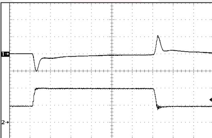
Figure 11: Output voltage response to step-change in load current 50%-100%-50% of Iout (max). Load cap: 1 µF ceramic cap and 10 µF, 100 mΩ ESR tantalum cap. Ch 1: Vout (300 mV/div). Ch 2: Iout (10 A/div). Horizontal Timescale: 100 µsec/div.
