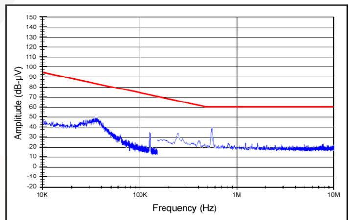
Figure 24: High frequency conducted emissions of MQFL-28-05S, 5 Vout module at 120 W output with MQME-28-P filter, as measured with Method CE102. Limit line shown is the 'Basic Curve' for all applications with a 28 V source.
