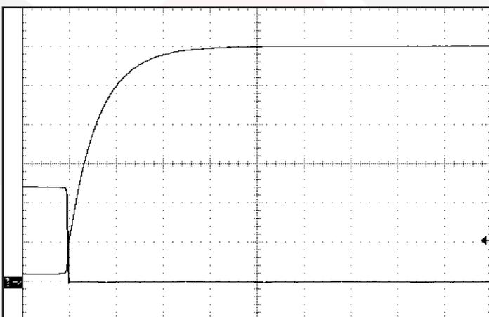
Figure 17: Rise of output voltage after the removal of a short circuit across the output terminals. Ch 1:  $V_{out}$  (1 V/div). Ch 2:  $I_{out}$  (10 A/div). Horizontal Timescale: 5 msec/div.
