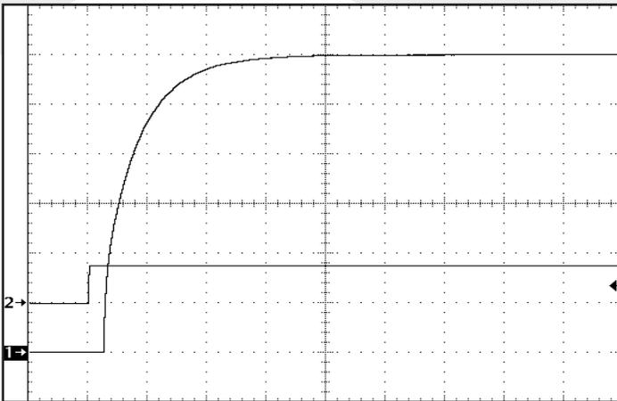
Figure 9: Turn-on transient at full resistive load and zero output capacitance initiated by ENA2. Input voltage pre-applied. Ch 1: Vout (1 V/div). Ch 2: ENA2 (5 V/div). Horizontal Timescale: 5 msec/div.
