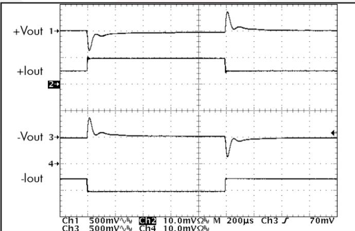
**Figure 17:** Output voltage response to step-change in total load current (50%-100%-50%) of total Iout (max) split 50%/50%. Load cap: 1µF ceramic cap and 10µF, 100 mΩ ESR tantalum cap. Ch 1: +Vout (500mV/div); Ch 2: +Iout (5A/div); Ch 3: -Vout (500mV/div); Ch 4: -Iout (5A/div).
