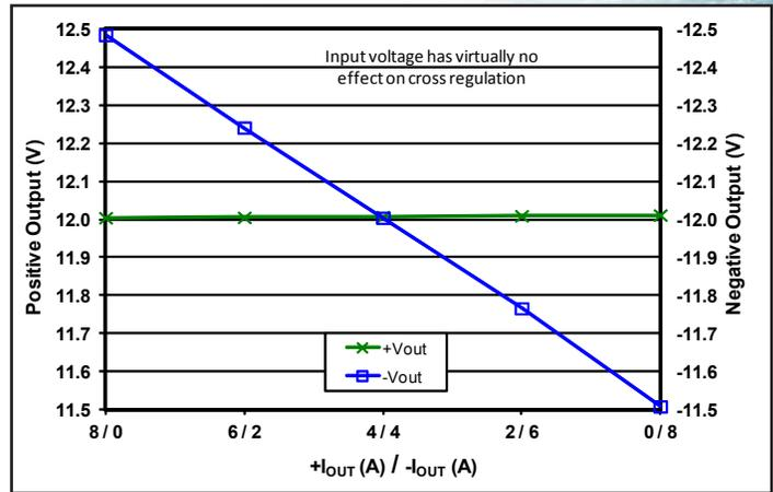
Figure 8: Load regulation vs. load current with power fixed at 80% load (96W) and load currents split as shown between the +12V and -12V outputs, at nominal input voltage and T<sub>case</sub> = 25°C.
