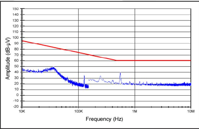
**Figure 33:** High frequency conducted emissions of MQFL-28-05S, 5Vout module at 120W output with MQME-28-P filter, as measured with Method CE102. Limit line shown is the 'Basic Curve' for all applications with a 28V source.
