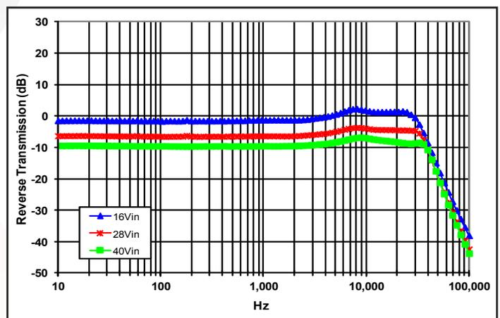
**Figure 29:** Magnitude of incremental reverse transmission from +12V output (+RT = iin /+iout) for minimum, nominal, and maximum input voltage at full rated power.
