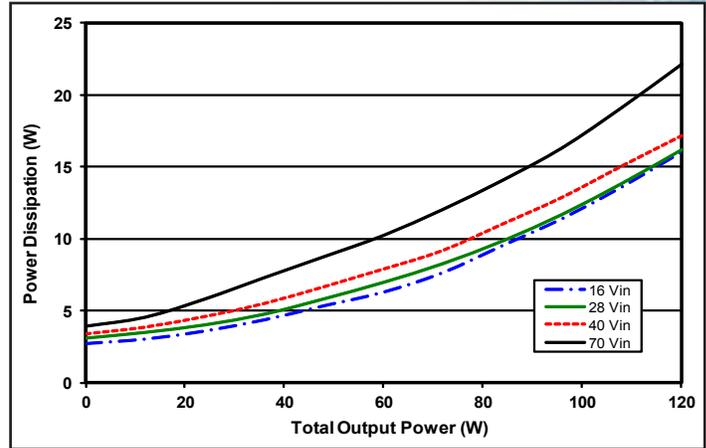
**Figure 2:** Power dissipation vs. output power, from zero load to full load with equal load on the +12V and -12V outputs at minimum, nominal, and maximum input voltage at 25°C.
