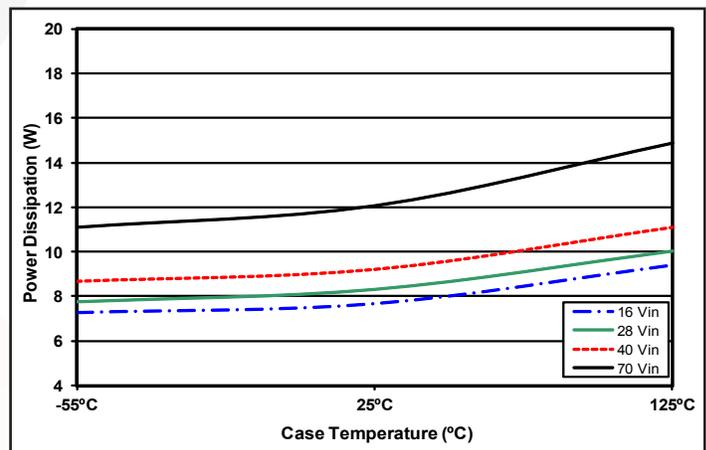
**Figure 6:** Power dissipation at 60% load (3A load on +12V and 3A load on -12V) versus case temperature for Vin = 16V, 28V, and 70V.
