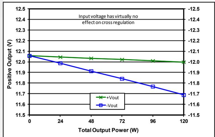
Figure 10: Load regulation vs. total output power from zero to full load where -I<sub>OUT</sub> equals three times +I<sub>OUT</sub> at nominal input voltage and T<sub>case</sub> = 25°C.
