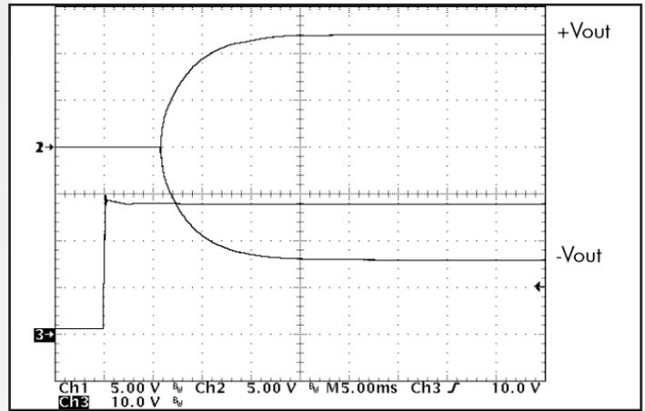
**Figure 16:** Turn-on transient at full load, after application of input voltage (ENA 1 and ENA 2 logic high) (5ms/div). Ch 1: +Vout (5V/div); Ch 2: -Vout (5V/div); Ch 3: Vin (10V/div).
