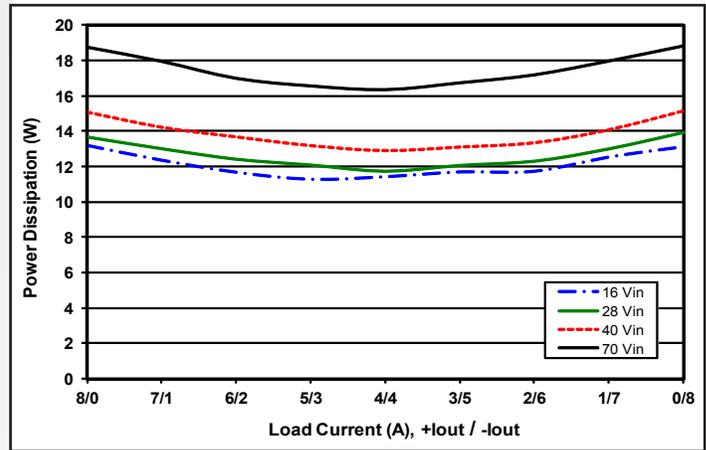
**Figure 4:** Power dissipation vs. output current, with total output current fixed at 80% load (96W) and loads split as shown between the +12V and -12V outputs at minimum, nominal, and max input voltage at 25°C.
