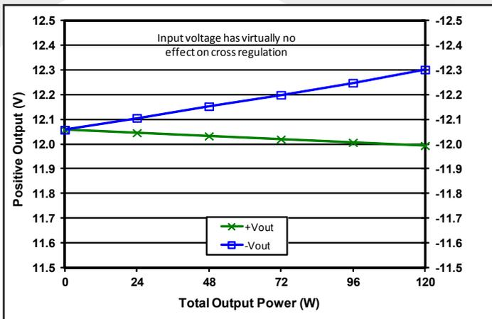
Figure 9: Load regulation vs. total output power from zero to full load where +I<sub>OUT</sub> equals three times -I<sub>OUT</sub> at nominal input voltage and T<sub>case</sub> = 25°C.
