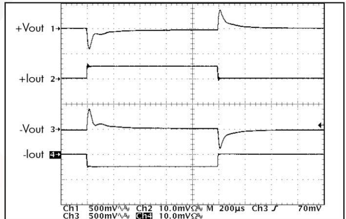
**Figure 18:** Output voltage response to step-change in total load current (0%-50%-0%) of total Iout (max) split 50%/50%. Load cap: 1µF ceramic cap and 10µF, 100 mΩ ESR tantalum cap. Ch 1: +Vout (500mV/div); Ch 2: +Iout (5A/div); Ch 3: -Vout (500mV/div); Ch 4: -Iout (5A/div).
