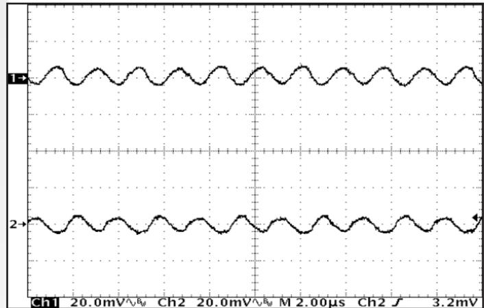
**Figure 22:** Output voltage ripple, +Vout (Ch 1) and -Vout (Ch 2), at nominal input voltage and full load current evenly split (20mV/div). Load capacitance: 1µF ceramic cap and 10µF tantalum cap. Bandwidth: 10MHz. See Figure 20.
