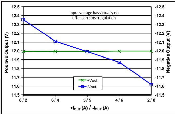
Figure 7: Load regulation vs. load current with power fixed at full load (120W) and load currents split as shown between the +12V and -12V outputs, at nominal input voltage and T<sub>case</sub> = 25°C.
