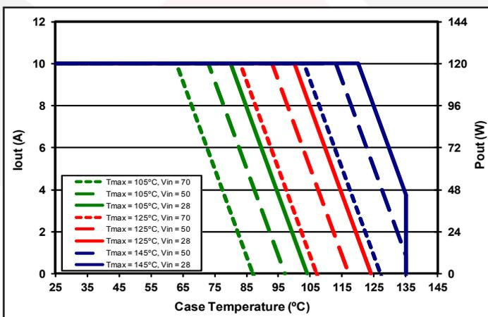
Figure 11: Total Output Current / Total Output Power derating curve as a function of T<sub>case</sub> and the maximum desired power MOSFET junction temperature (see Note 15).
