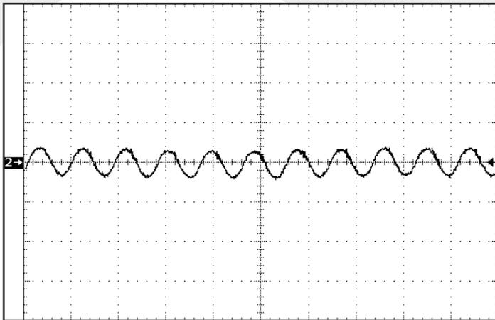
Figure 15: Input terminal current ripple,  $i_c$ , at full rated output current and nominal input voltage with SynQor MQ filter module (50mA/div). Horizontal Timescale: 2 $\mu$ sec/div. Bandwidth: 20MHz. See Figure 14.
