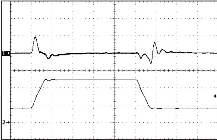
Figure 13: Output voltage response to step-change in input voltage (16V-50V-16V). Load cap: 10 $\mu$ F, 100m $\Omega$  ESR tantalum cap and 1 $\mu$ F ceramic cap. Ch 1:  $V_{out}$  (200mV/div). Ch 2:  $V_{in}$  (20V/div). Horizontal Timescale: 200 $\mu$ sec/div.
