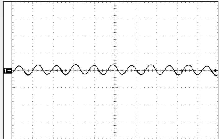
Figure 16: Output voltage ripple,  $V_{out}$ , at nominal input voltage and rated load current (20mV/div). Load capacitance: 1 $\mu$ F ceramic capacitor and 10 $\mu$ F tantalum capacitor. Horizontal Timescale: 2 $\mu$ sec/div. Bandwidth: 10MHz. See Figure 14.
