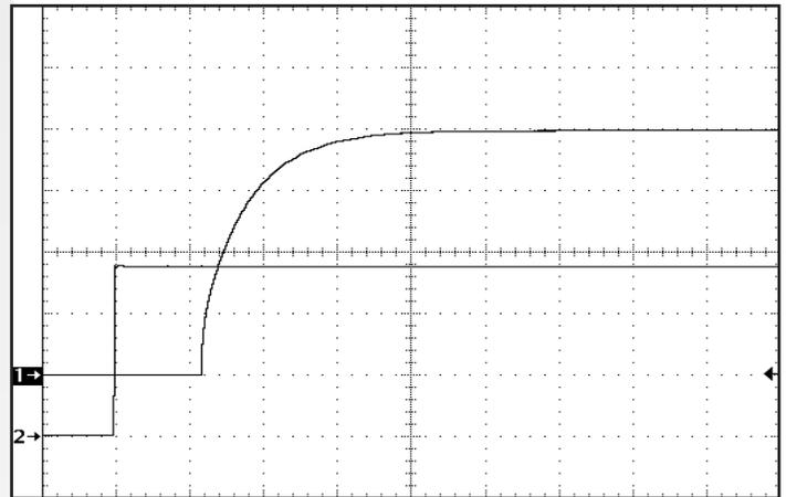
Figure 10: Turn-on transient at full resistive load and zero output capacitance initiated by Vin. ENA1 and ENA2 both previously high. Ch 1: Vout (3V/div). Ch 2: Vin (10V/div). Horizontal Timescale: 5msec/div.
