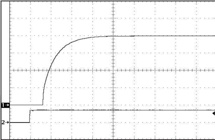
Figure 7: Turn-on transient at full resistive load and zero output capacitance initiated by ENA1. Input voltage pre-applied. Ch 1: Vout (3V/div). Ch 2: ENA1 (5V/div). Horizontal Timescale: 5msec/div.
