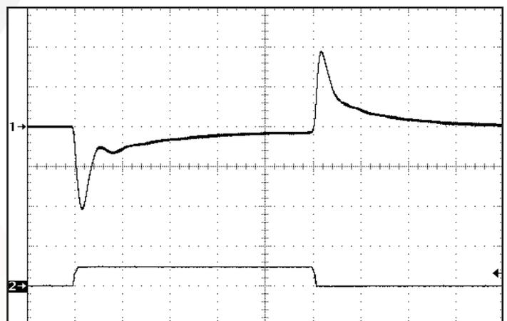
Figure 12: Output voltage response to step-change in load current 0%-50%-0% of Iout (max). Load cap: 1µF ceramic cap and 10µF, 100mΩ ESR tantalum cap. Ch 1: Vout (200mV/div). Ch 2: Iout (10A/div). Horizontal Timescale: 100µsec/div.
