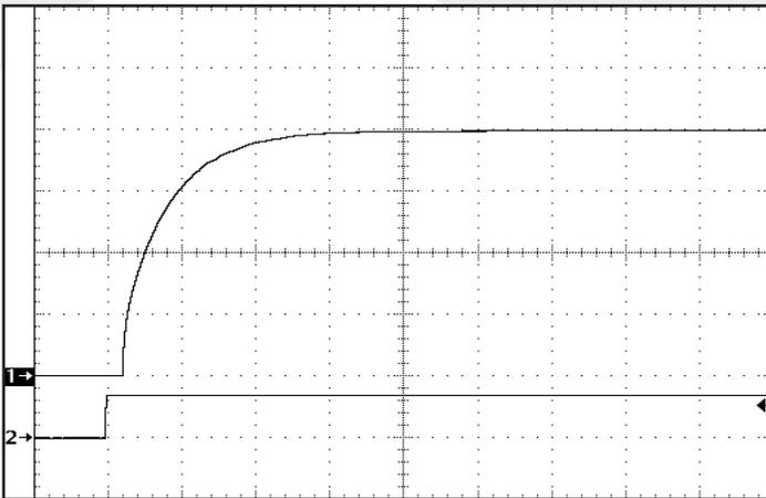
Figure 9: Turn-on transient at full resistive load and zero output capacitance initiated by ENA2. Input voltage pre-applied. Ch 1: Vout (3V/div). Ch 2: ENA2 (5V/div). Horizontal Timescale: 5msec/div.
