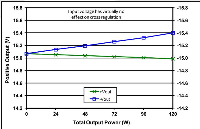
Figure 9: Load regulation vs. total output power from zero to full load where +Iout equals three times -Iout at nominal input voltage and Tcase = 25°C.
