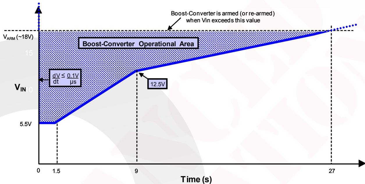
Under-Voltage Transient Profile showing when the boost-converter is guaranteed to be operational. Before the boost converter will operate, it must first be armed (or re-armed) by making  $V_{IN}$  greater than  $V_{ARM}$ .
