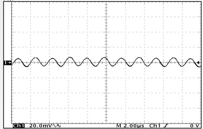
Figure 16: Output voltage ripple,  $V_{out}$ , at nominal input voltage and rated load current (20mV/div). Load capacitance: 1 $\mu$ F ceramic capacitor and 10 $\mu$ F tantalum capacitor. Bandwidth: 10MHz. See Figure 14.
